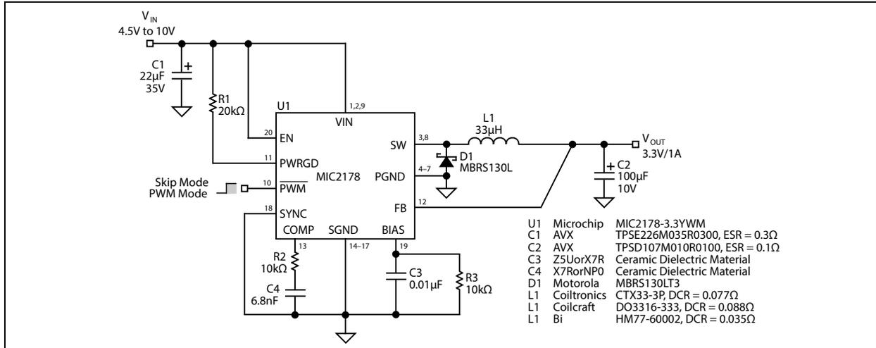
**FIGURE 5-5:** MIC2178 4.5V - 10V to 3.3V/1A Regulator.
