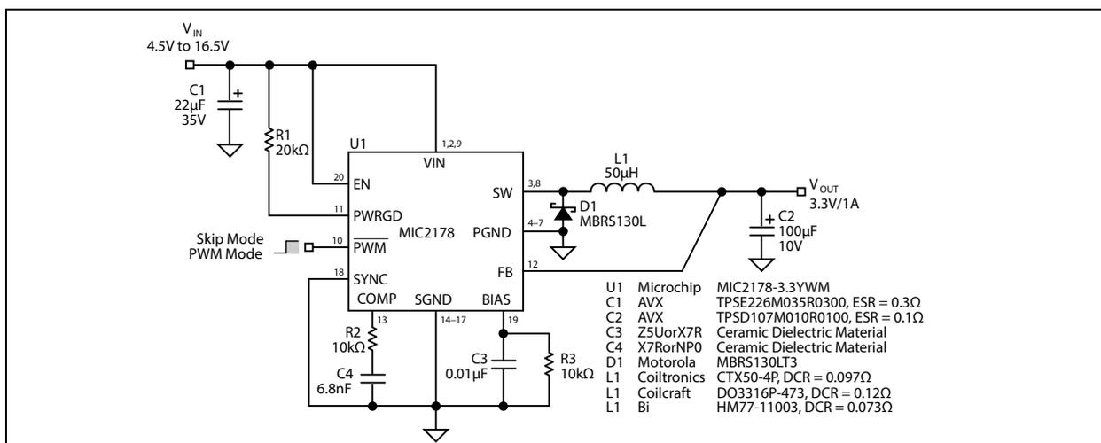
**FIGURE 5-1:** MIC2178 4.5V - 16.5V to 3.3V/1A Regulator.
