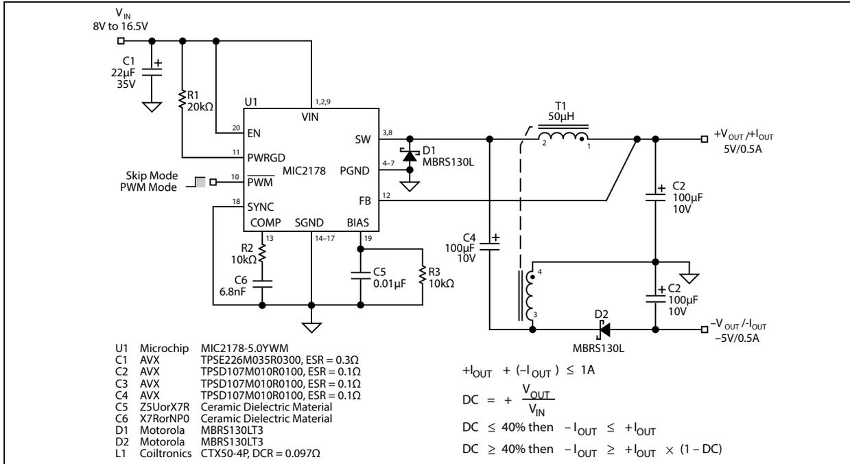
**FIGURE 5-7:** MIC2178 8V - 16.5V to ±5V/500 mA Regulator.
