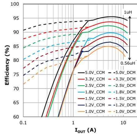
Figure 26: XR76112, 12V<sub>IN</sub>, 600kHz
