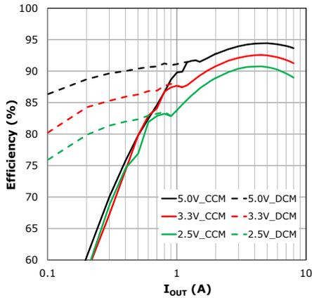
Figure 27: XR76108, 22V<sub>IN</sub>, 400kHz, 3.3µH
