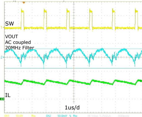
Figure 7: XR76112  $V_{OUT}$  Ripple is 14mV at 12A
