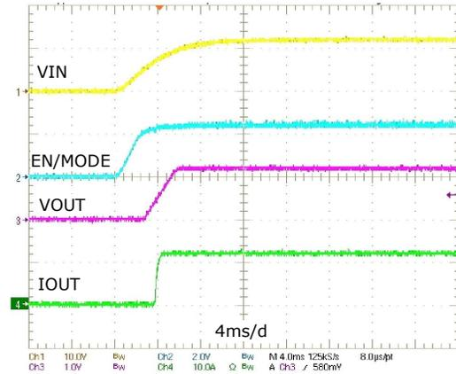
Figure 18: XR76112 Power-up, Forced CCM,  $I_{OUT} = 12A$
