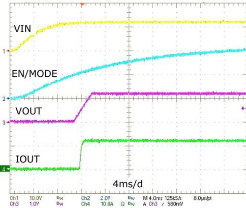
Figure 20: XR76112 Power-up, DCM / CCM,  $I_{OUT} = 12A$
