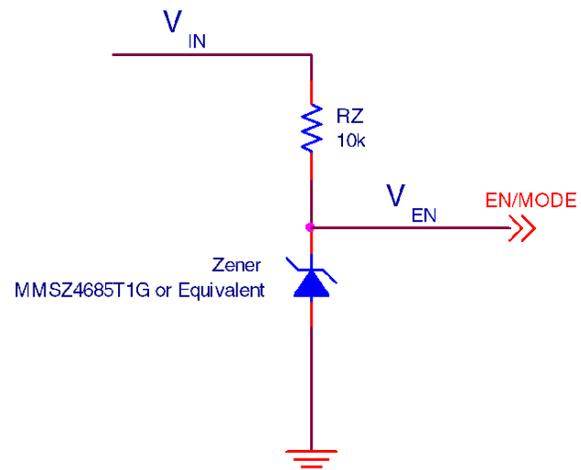
Figure 34: Selecting DCM/CCM by Deriving EN/MODE from  $V_{IN}$
