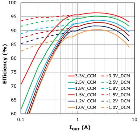
Figure 23: XR76108, 5V<sub>IN</sub>, 600kHz, 1µH
