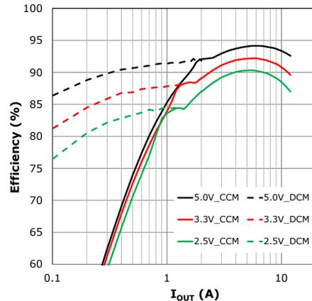
Figure 28: XR76112, 22V<sub>IN</sub>, 400kHz, 2.2µH
