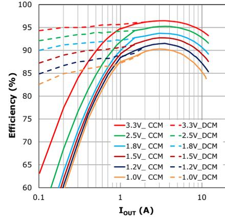
Figure 24: XR76112, 5V<sub>IN</sub>, 600kHz, 0.56µH
