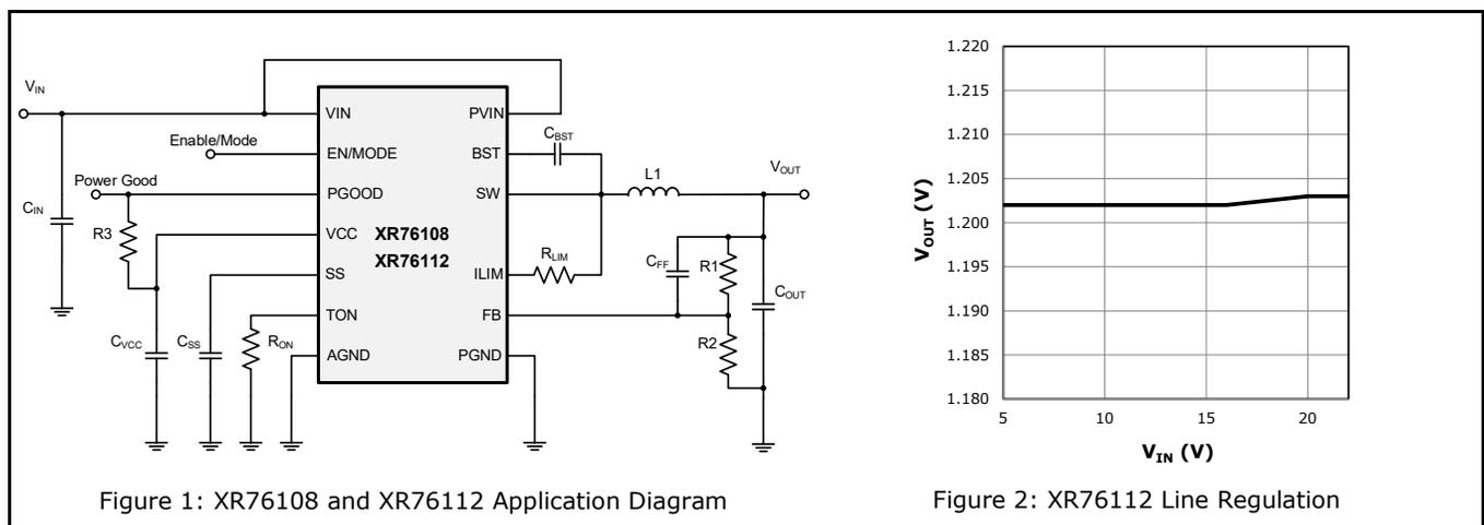
Figure 1: XR76108 and XR76112 Application Diagram
