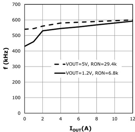
Figure 9: XR76112 Frequency vs.  $I_{OUT}$ , Forced CCM
