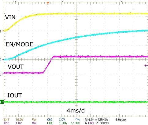
Figure 19: XR76112 Power-up, DCM / CCM,  $I_{OUT} = 0A$
