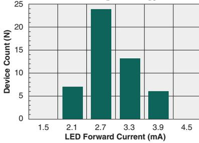
**Typical  $I_F$  for Switch Dropout**
