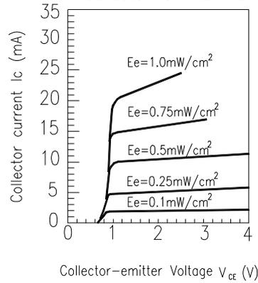
**Typical Electrical/Optical/Characteristics Curves for ITR**
