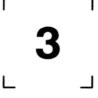
3   | Transmission — Forward Third Gear<br>Use sequential numbers as needed<br>for additional forward gears: 4 for<br>fourth gear, etc.          | None | ISO 3767-1<br>ISO 6405-1<br>ISO 7296-2 |
