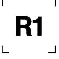
R1 | Transmission — Reverse First Gear<br>Use sequential numbers as needed<br>for additional reverse gears: R2 for<br>reverse second gear, etc. | None | ISO 3767-1<br>ISO 6405-1<br>ISO 7296-2 |
