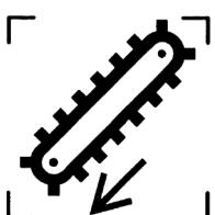
A schematic diagram of a scraper elevator. It shows a horizontal bar with a series of vertical segments representing tines or blades. An arrow points downwards along the length of the bar, indicating the direction of material flow or卸载 (unload). | Scraper Elevator — Unload | 1535 | ISO 6405-2 |
