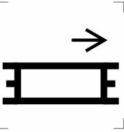
A schematic diagram of a compactor machine. It features a central rectangular body with two side supports. A horizontal arrow pointing to the right is positioned above the machine, indicating the direction of side shift. | <b>Compactor — Side Shift Right</b> | None | — |
