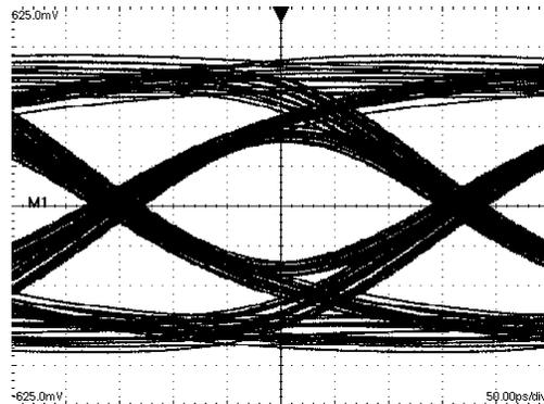
**Figure 19. An Equalized (with PE) 3.125 Gbps NRZ PRBS-7 After 40" Differential FR-4 Stripline
