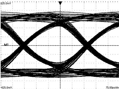
**Figure 18. An Equalized (with PE) 2.5 Gbps NRZ PRBS-7 After 40" Differential FR-4 Stripline
