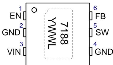
Figure 2 - Pinout UDFN 2x2 6L Top View
