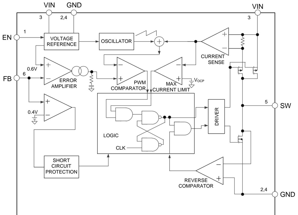
Figure 3 - Simplified Block Diagram of LX7188
