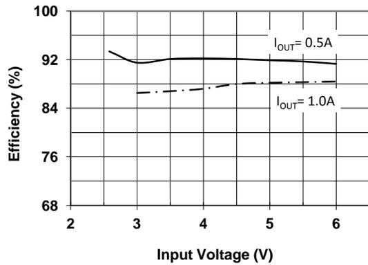
Figure 6 · Efficiency vs. Input Voltage
