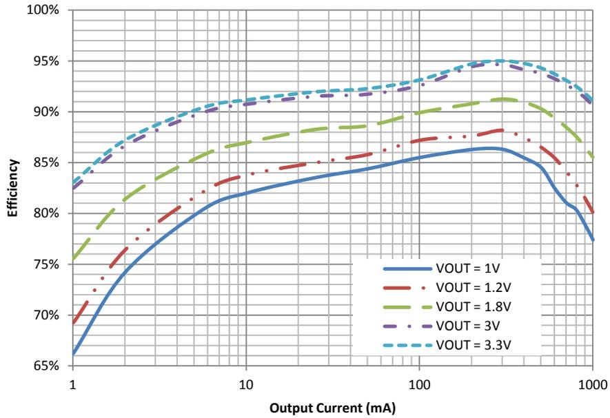
Figure 4 · Efficiency vs. Output Current with 5V Input
