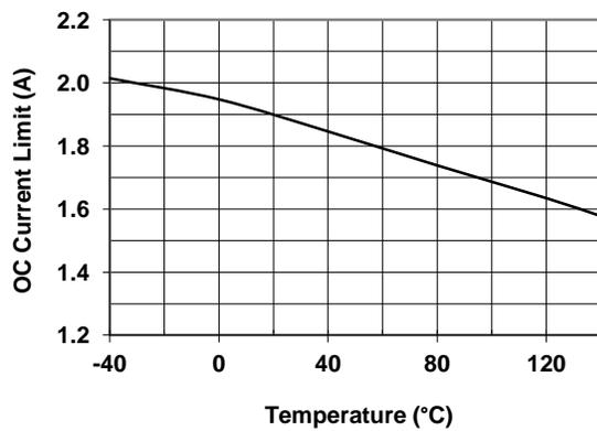
Figure 10 · OCP Current Limit vs. Temperature
