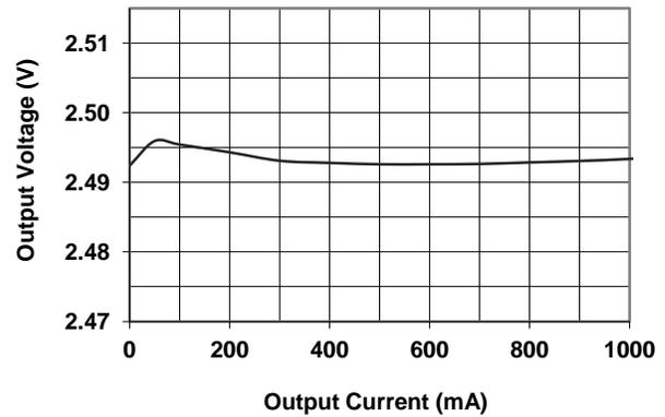
Figure 7 · Output Voltage vs. Output Current
