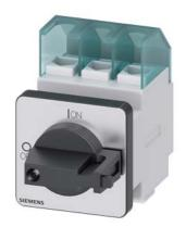
SENTRON, Switch disconnector 3LD, main switch, 3-pole, lu: 25 A, Operating power / at AC-23 A at 400 V: 9.5 kW, floor mounting with door coupling, knob-operated mechanism, black, 4-hole mounting of the handle
