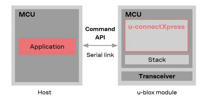
Architecture of a mesh node using u-connectXpress
