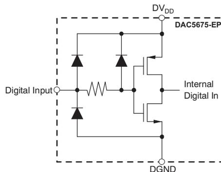
**Figure 15. CMOS/TTL Digital Equivalent Input**
