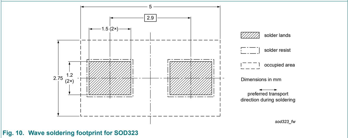
**Fig. 10. Wave soldering footprint for SOD323**
