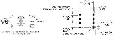
Application of the transformer allows for the leadwires between terminals 1&2 and 3&4 to solder bridge.
