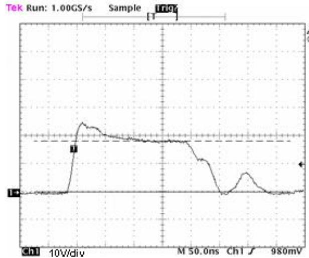
Figure 6. SMS15CT1 ESD Response for IEC 61000-4-2 (+8.0 kV Contact)
