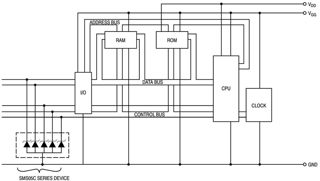
Figure 8. Microprocessor Protection
