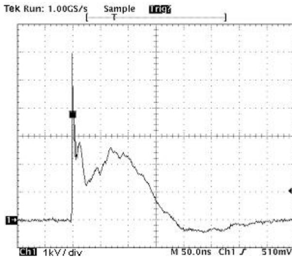
Figure 5. ESD Pulse IEC 61000-4-2 (8.0 kV Contact)
