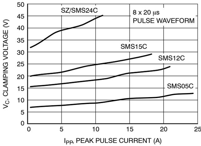
Figure 3. Clamping Voltage vs. Peak Pulse Current
