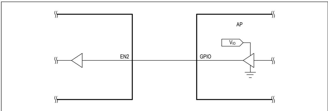
Figure 22. EN2 Simplified Input Stage: Active-High or Low
