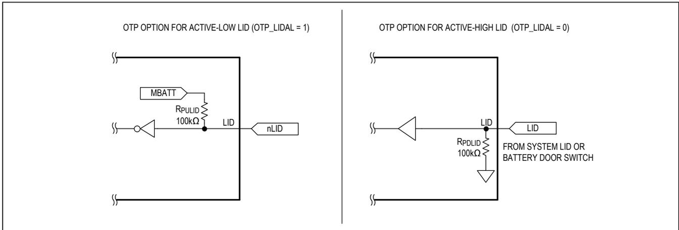
Figure 24. LID Simplified Input Stage: Active-High or Low
