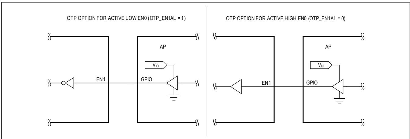
Figure 21. EN1 Simplified Input Stage: Active-High or Low
