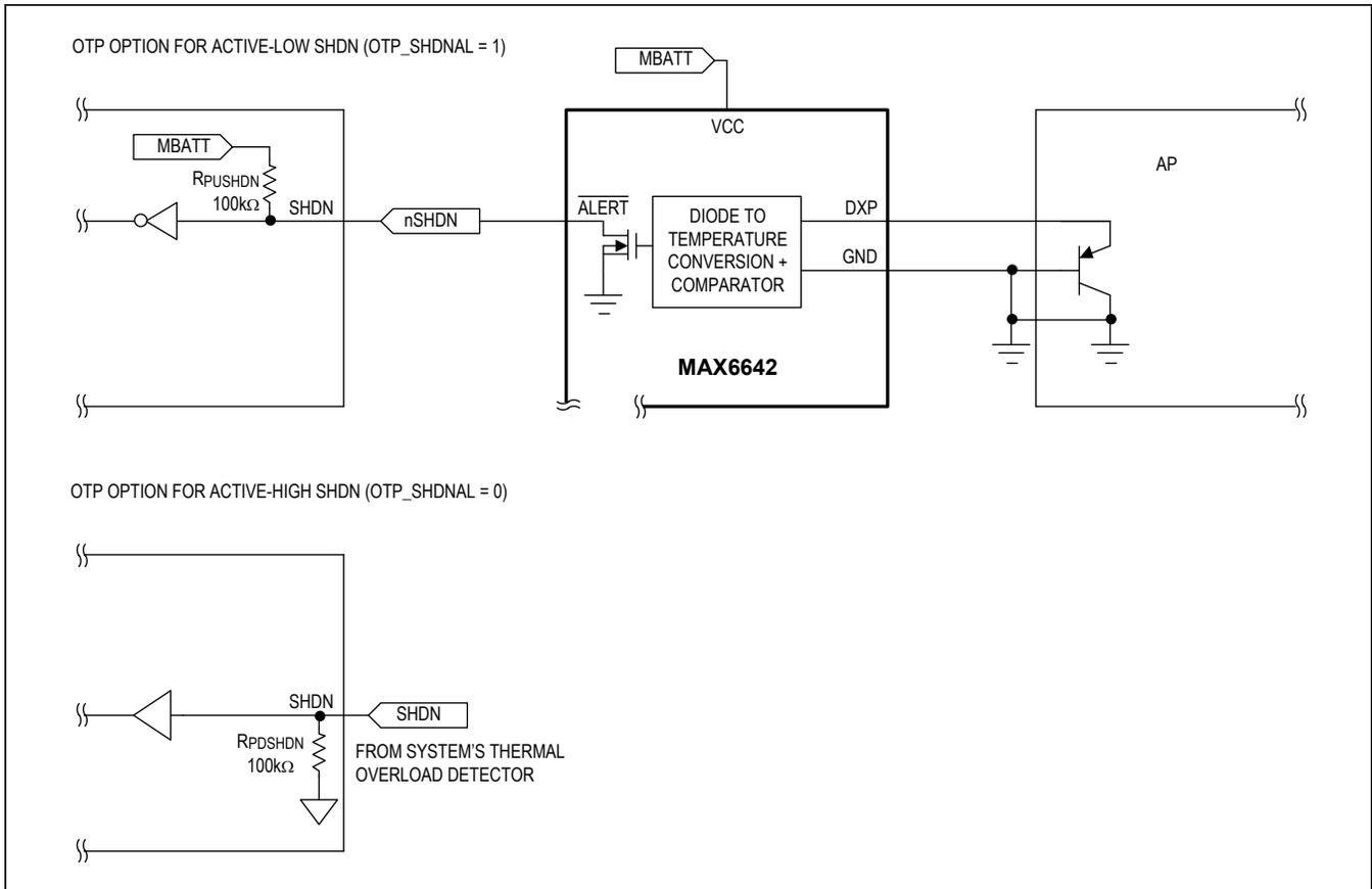
Figure 25. SHDN Simplified Input Stage: Active-High or Low
