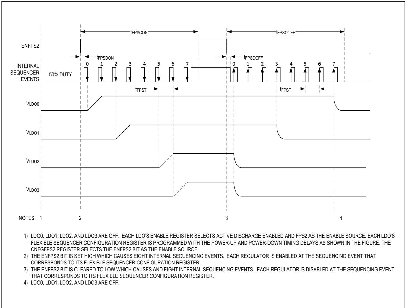
Figure 28. Example Timing Diagram: Flexible Power Sequencer
