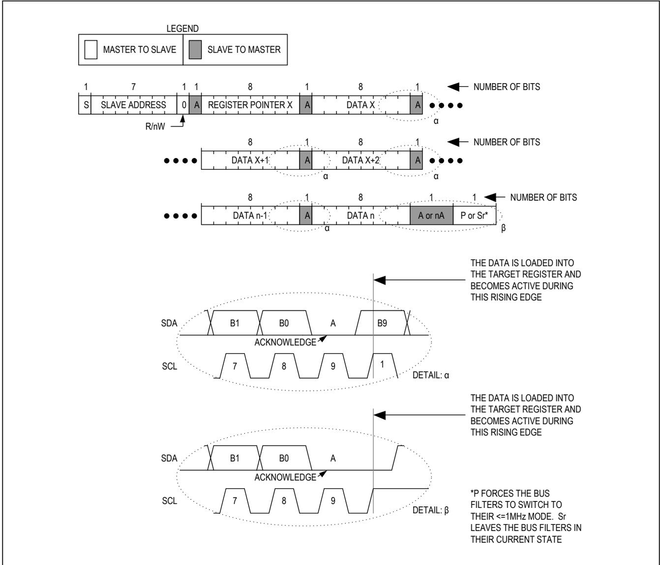
Figure 35. Writing to Sequential Register "x" to "n"
