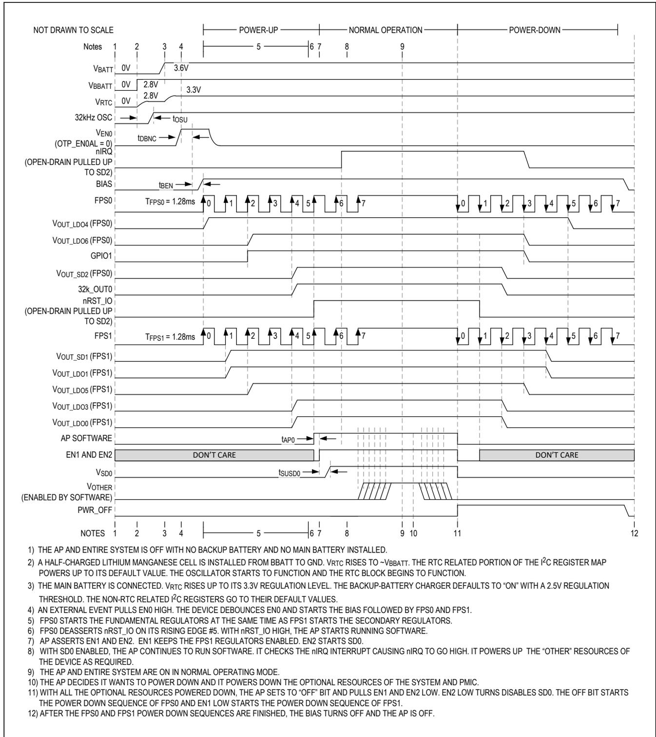
Figure 26. Application Processor Power-Up and Power-Down Timing
