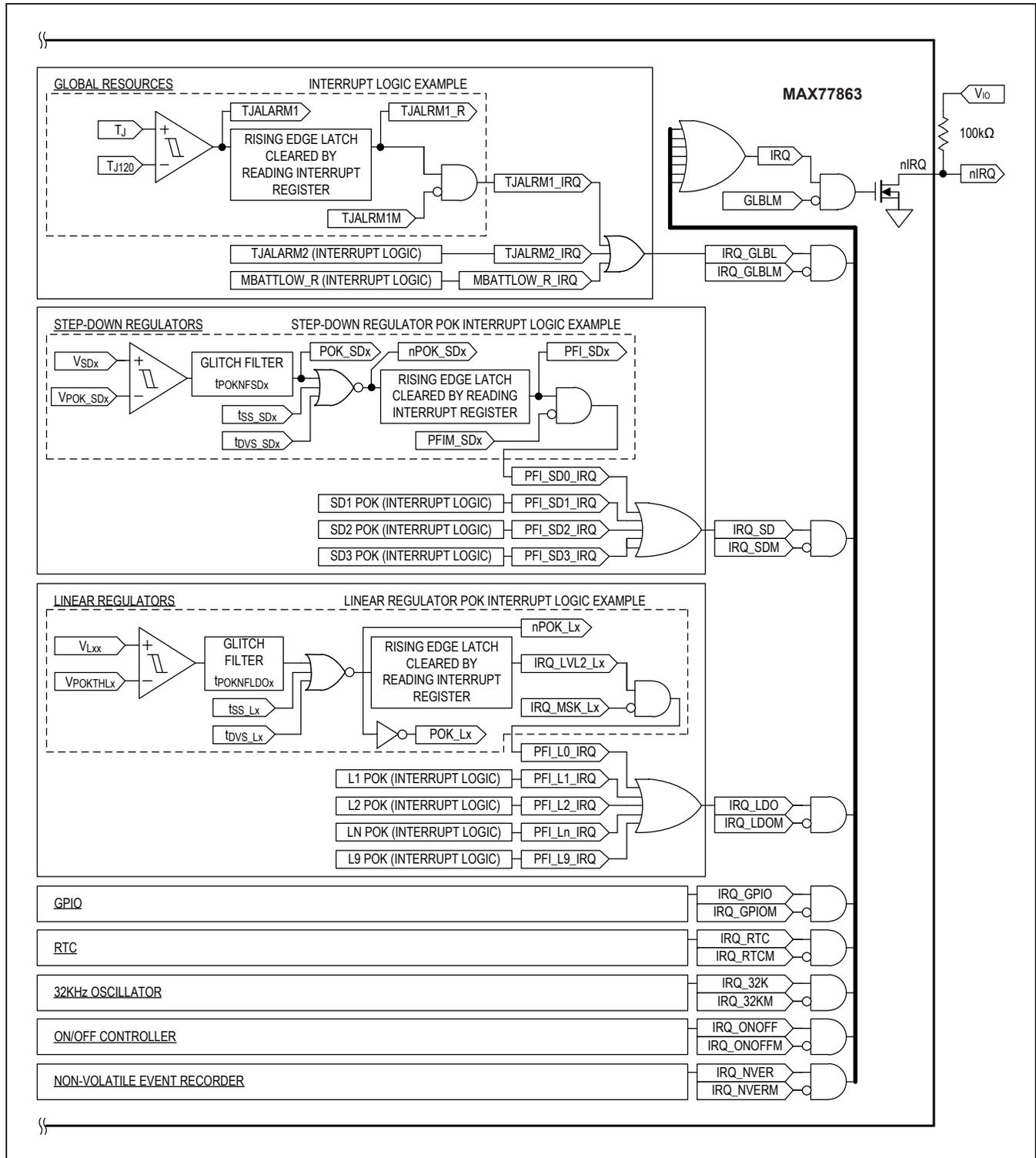
Figure 2. Simplified Interrupt, Status, and Mask Logic
