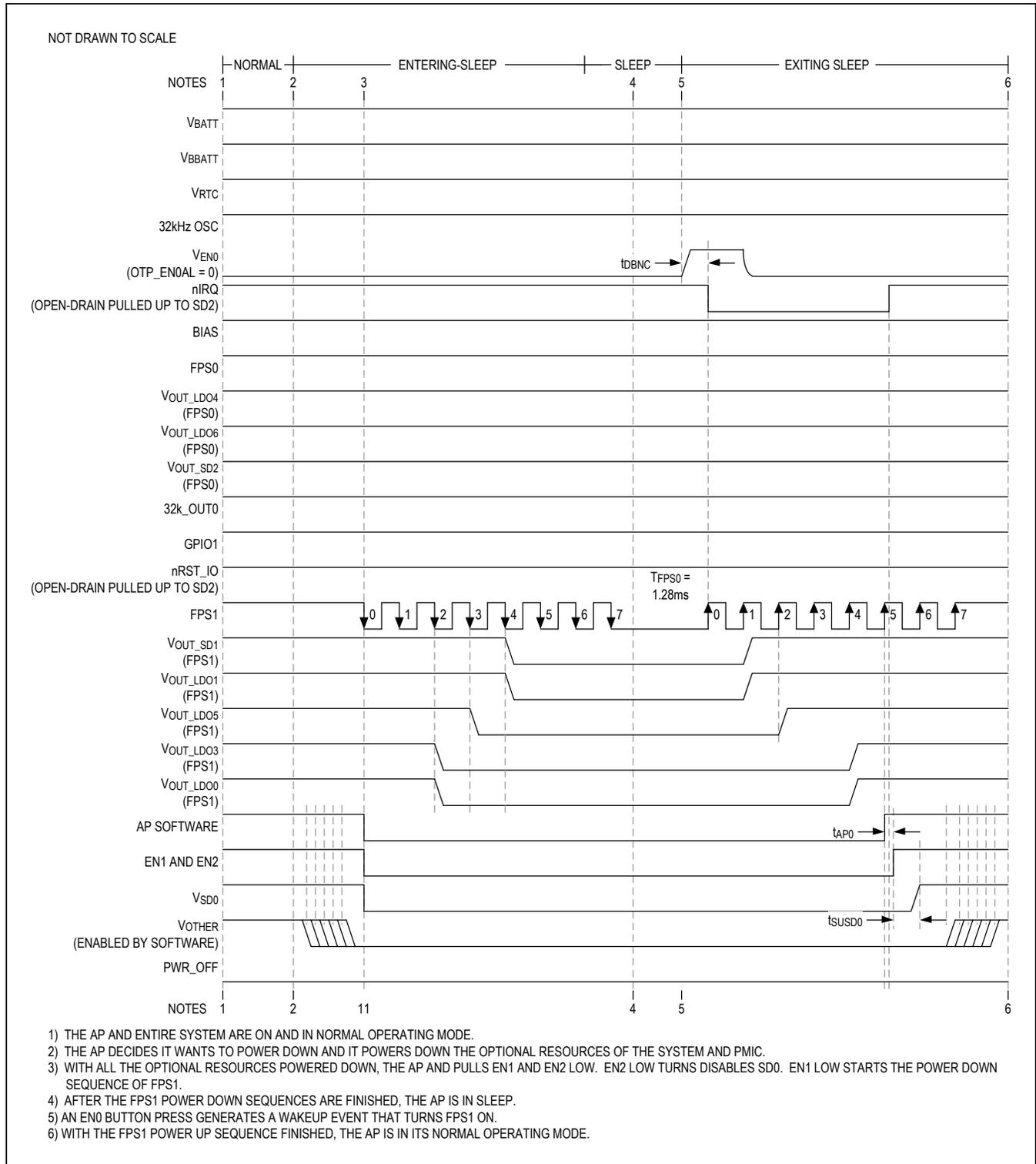
Figure 27. Application Processor Entering and Exiting Sleep Timing
