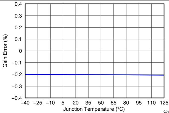
Figure 17. Rx PGA2 Gain Error vs Temperature
