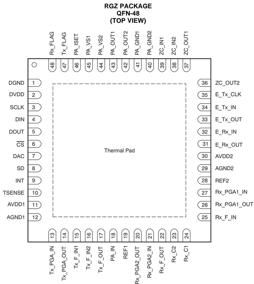
NOTE: Exposed thermal pad is connected to ground.
