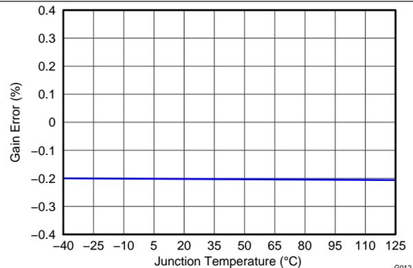
Figure 16. Rx PGA1 Gain Error vs Temperature
