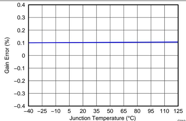
Figure 14. Tx PGA Gain Error vs Temperature
