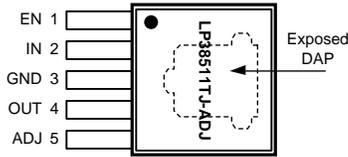
**Figure 1. 5-Pin PFM, Top View**
