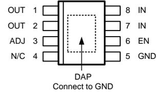
**Figure 2. 8-Pin SO PowerPad, Top View**
