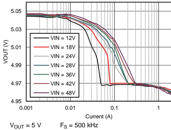
Figure 9.  $V_{OUT}$  Regulation
