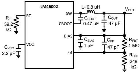
$V_{OUT} = 5\text{ V}$   $F_S = 1\text{ MHz}$   $V_{IN} = 24\text{ V}$
