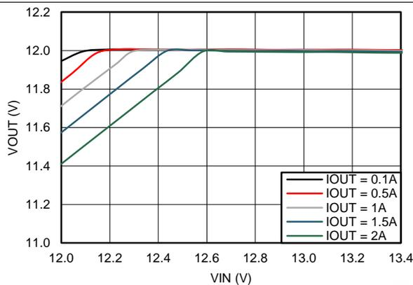
Figure 17. Dropout Curve
