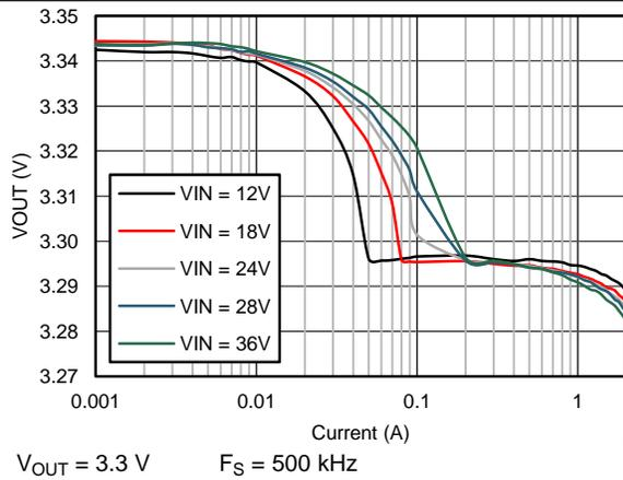
Figure 7.  $V_{OUT}$  Regulation
