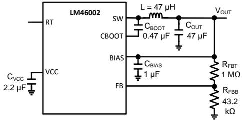
$V_{OUT} = 24\text{ V}$   $F_S = 500\text{ kHz}$   $V_{IN} = 48\text{ V}$
