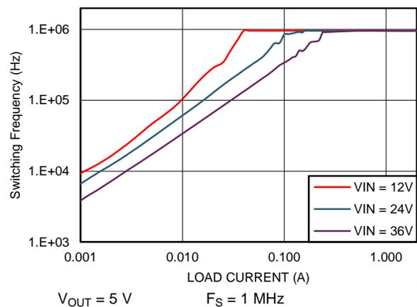
Figure 88. Switching Frequency vs  $I_{OUT}$  in PFM Operation
