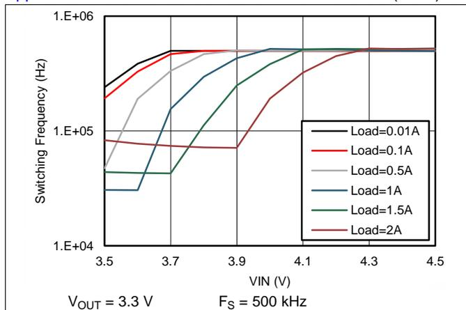
Figure 19. Switching Frequency vs  $V_{IN}$  in Dropout Operation
