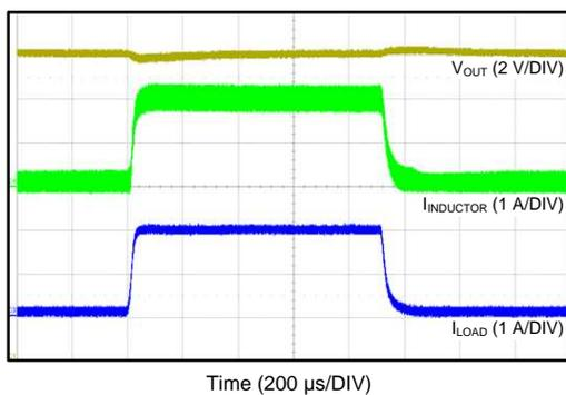
$V_{OUT} = 24\text{ V}$   $F_S = 500\text{ kHz}$   $V_{IN} = 48\text{ V}$
