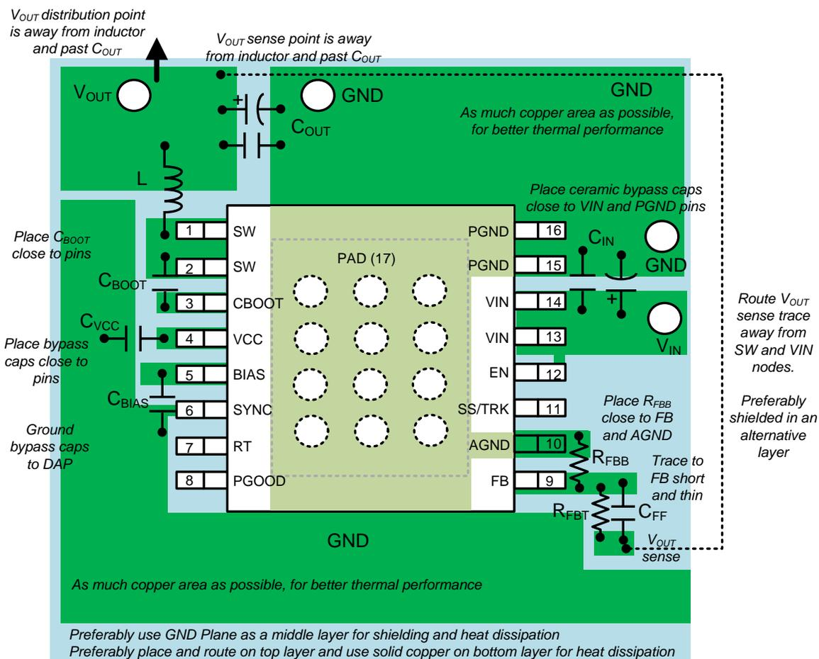
Figure 102. LM46002 PCB Layout Example and Guidelines
