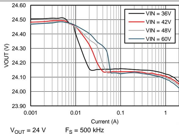
Figure 12.  $V_{OUT}$  Regulation
