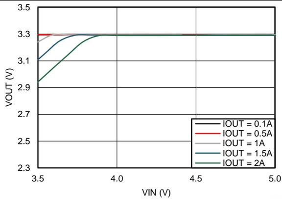
Figure 13. Dropout Curve
