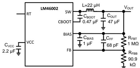
$V_{OUT} = 12\text{ V}$   $F_S = 500\text{ kHz}$   $V_{IN} = 24\text{ V}$
