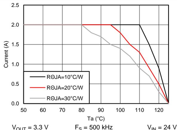
Figure 52. Derating Curve
