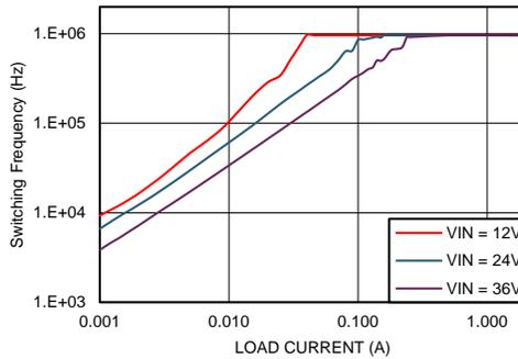
**Figure 34. Switching Frequency Decreases With Lower Load Current in PFM Operation**
