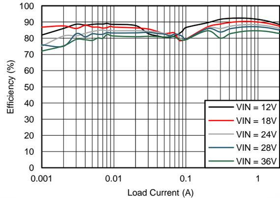
$V_{OUT} = 5\text{ V}$   $F_S = 500\text{ kHz}$
