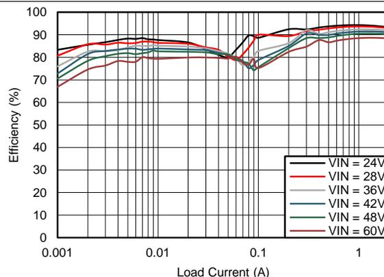
$V_{OUT} = 12\text{ V}$   $F_S = 500\text{ kHz}$
