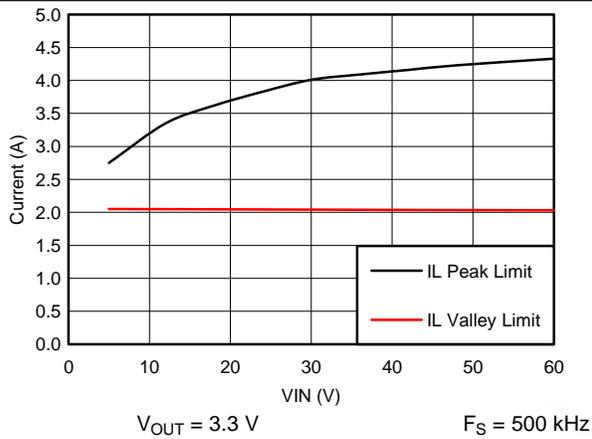
**Figure 31. Peak and Valley Current Limits vs  $V_{IN}$**
