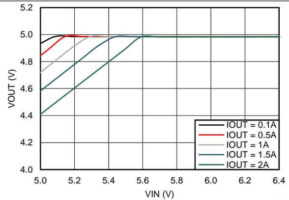
Figure 16. Dropout Curve
