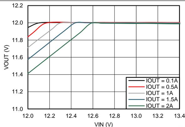
$V_{OUT} = 12\text{ V}$   $F_S = 500\text{ kHz}$
