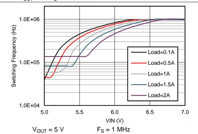
Figure 20. Switching Frequency vs  $V_{IN}$  in Dropout Operation
