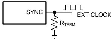
**Figure 41. Frequency Synchronization**
