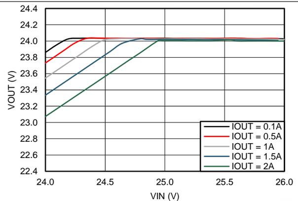
Figure 18. Dropout Curve
