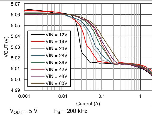
Figure 8.  $V_{OUT}$  Regulation
