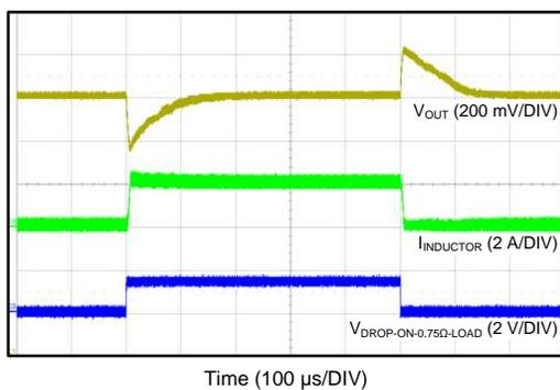
$V_{OUT} = 5\text{ V}$   $F_S = 1\text{ MHz}$   $V_{IN} = 24\text{ V}$
