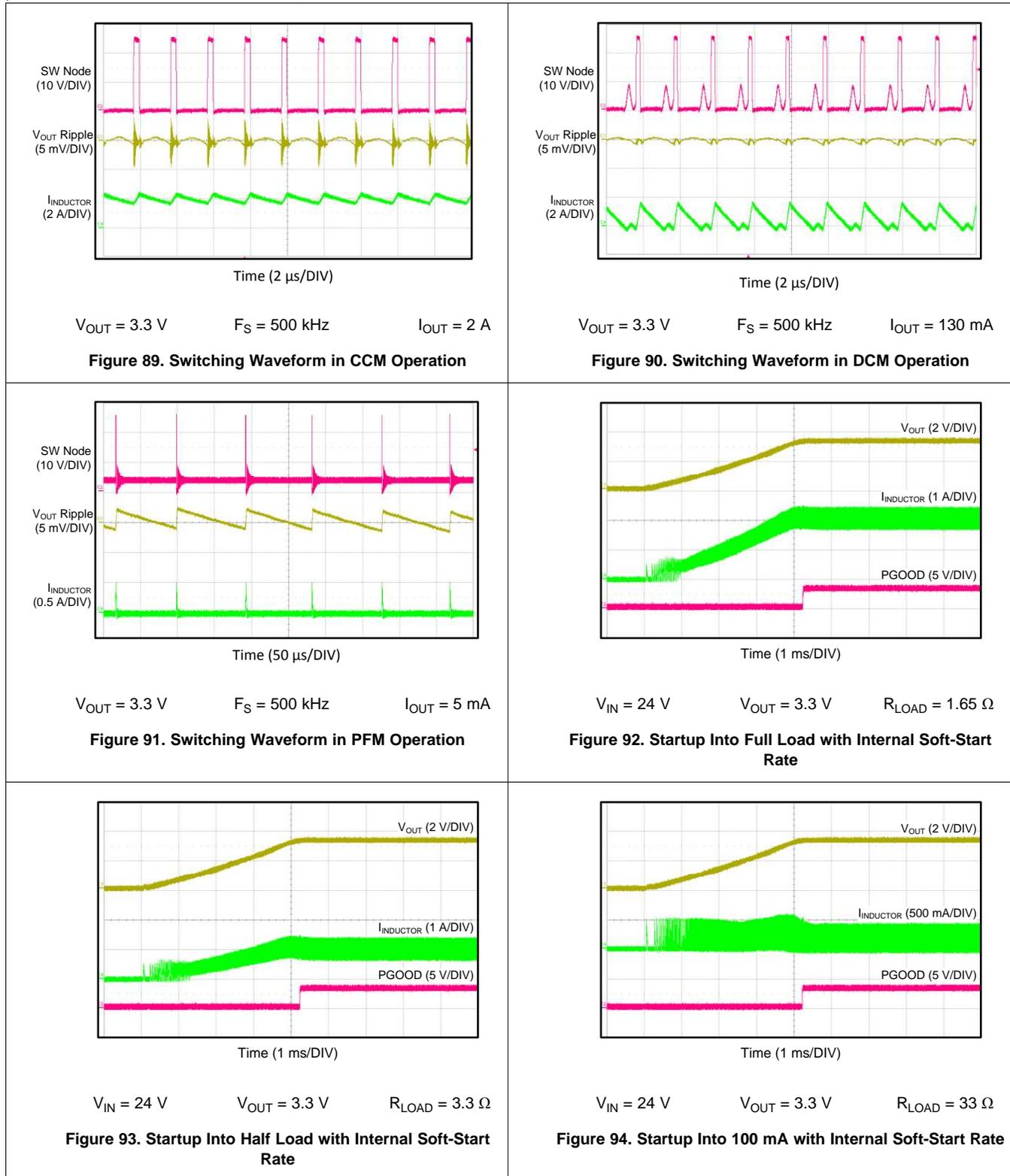
Please refer to Table 2 for bill of materials for each  $V_{OUT}$  and  $F_S$  combination. Unless otherwise stated, application performance curves were taken at  $T_A = 25\text{ }^\circ\text{C}$ .
