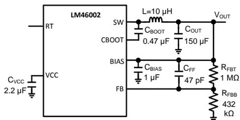
$V_{OUT} = 3.3\text{ V}$   $F_S = 500\text{ kHz}$   $V_{IN} = 24\text{ V}$
