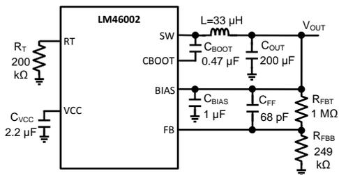
$V_{OUT} = 5\text{ V}$   $F_S = 200\text{ kHz}$   $V_{IN} = 24\text{ V}$
