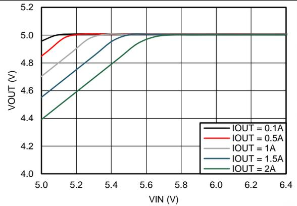
Figure 14. Dropout Curve
