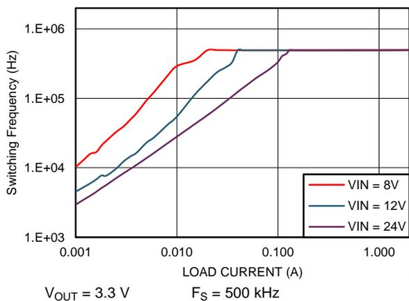
Figure 87. Switching Frequency vs  $I_{OUT}$  in PFM Operation
