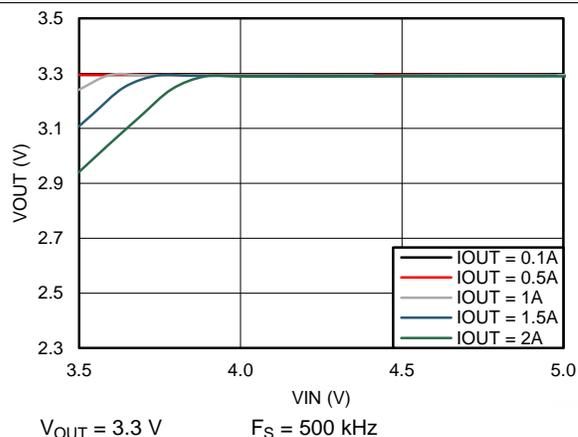
Figure 50. Drop-Out Curve
