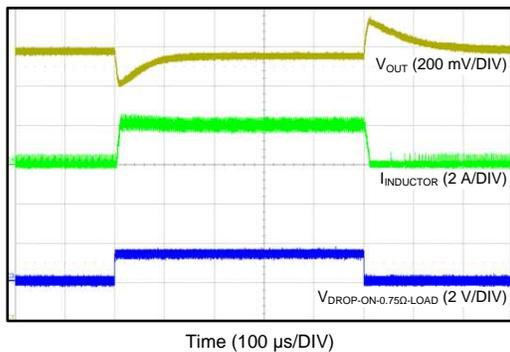
$V_{OUT} = 5\text{ V}$   $F_S = 500\text{ kHz}$   $V_{IN} = 24\text{ V}$
