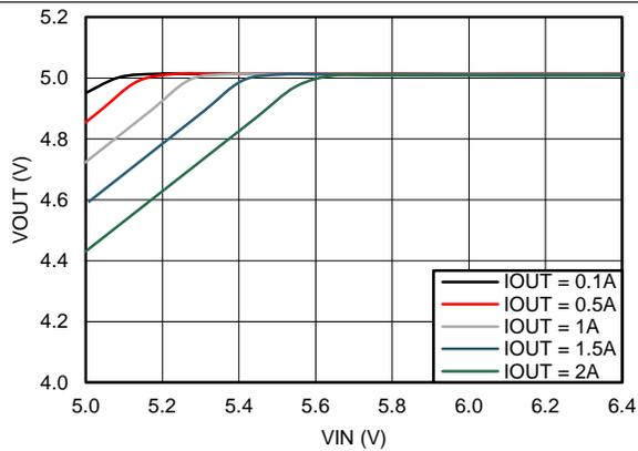
Figure 15. Dropout Curve
