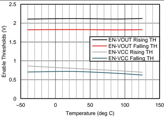
Figure 27. Enable Threshold vs Junction Temperature
