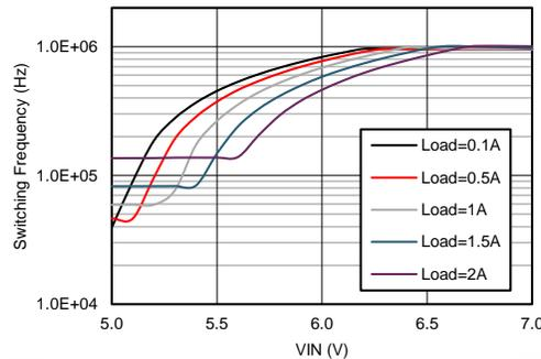
**Figure 42. Switching Frequency Decreases in Dropout Operation**
