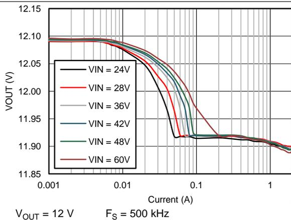
Figure 11.  $V_{OUT}$  Regulation
