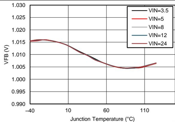
Figure 30. Feedback Voltage vs Junction Temperature
