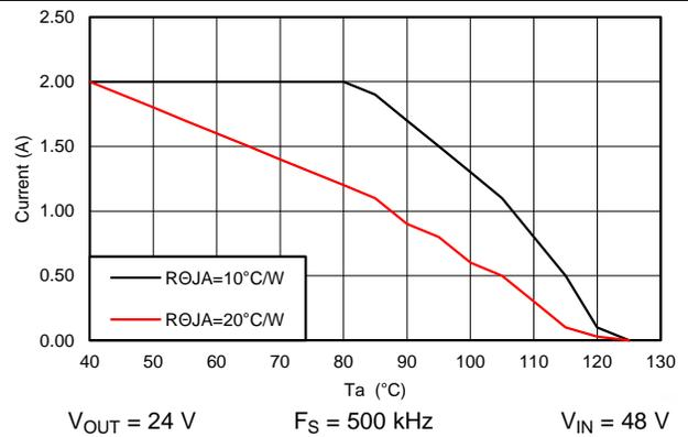
Figure 82. Derating Curve
