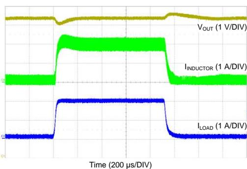
$V_{OUT} = 12\text{ V}$   $F_S = 500\text{ kHz}$   $V_{IN} = 24\text{ V}$
