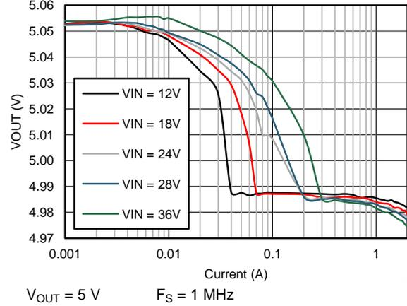
Figure 10.  $V_{OUT}$  Regulation
