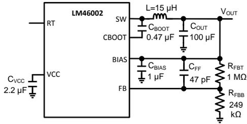
$V_{OUT} = 5\text{ V}$   $F_S = 500\text{ kHz}$   $V_{IN} = 24\text{ V}$
