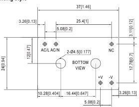
Case No.IRM03 Unit:mm[inch] Tolerance:±0.5[±0.02] unless otherwise specified
