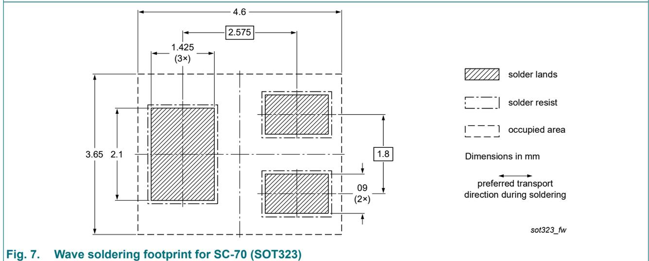
Fig. 7. Wave soldering footprint for SC-70 (SOT323)
