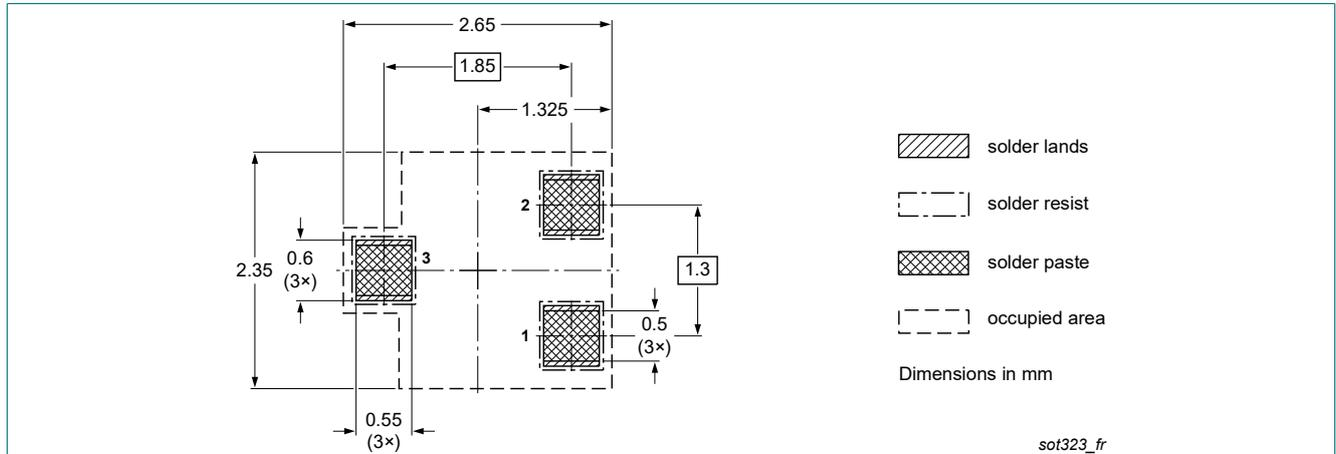
Fig. 6. Reflow soldering footprint for SC-70 (SOT323)
