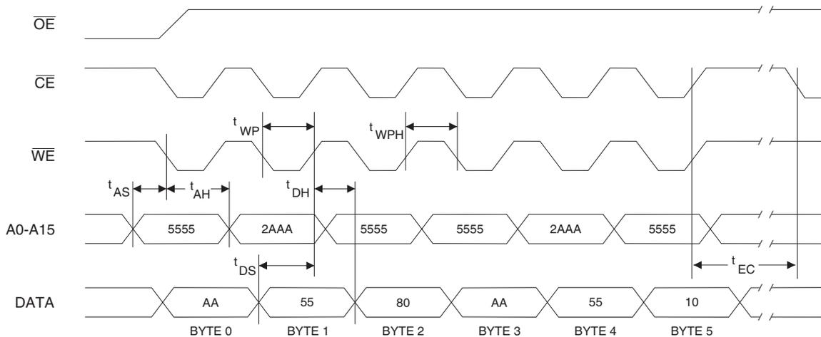
Note: 1.  $\overline{OE}$  must be high only when  $\overline{WE}$  and  $\overline{CE}$  are both low.
