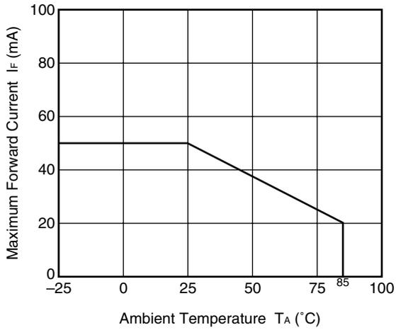
**MAXIMUM LOAD CURRENT vs. AMBIENT TEMPERATURE**
