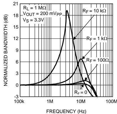
**Figure 28. Effect of Source Resistance on Peaking**
