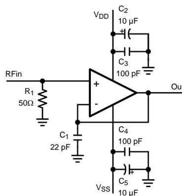
**Figure 31. Circuit for Coupling the RF Signal to IN+**
