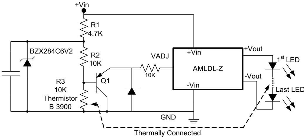
The selection of components for the thermal feedback circuit is depends on the choice of R2 and R3 and the effectiveness of the LED heatsink. To optimize the LED brightness control at high temperatures, the LEDs must have a sufficient thermal extraction path, if not the reduction in drive current will not be optimal.
