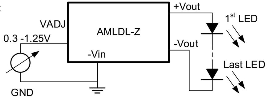
$$V_{ADJ} = \frac{R_2}{R_1 + R_2} \times V_{ctrl}$$
