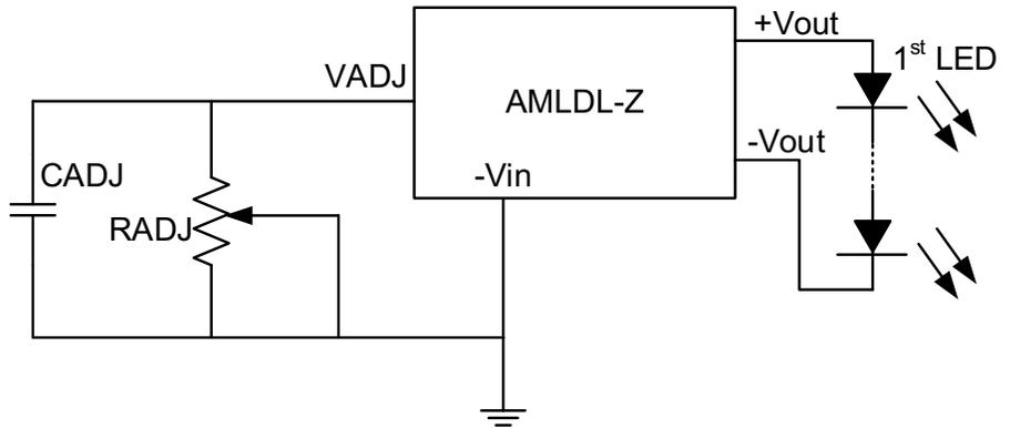
NOTE: Typical error is ±10% with resistive dimming control
