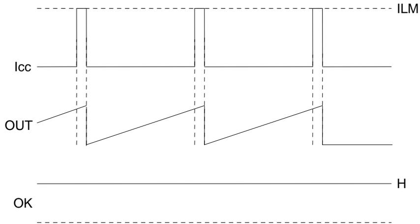
Fig. 20 Operation by current limit detection
