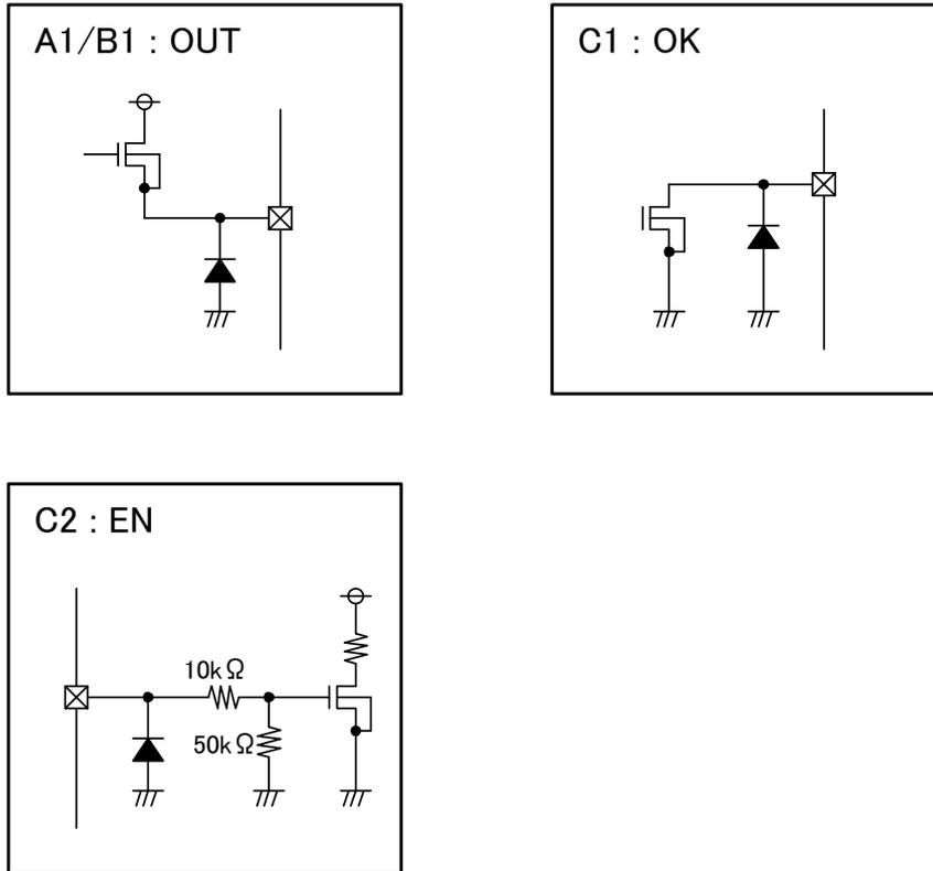
Fig. 16 Block Diagram
