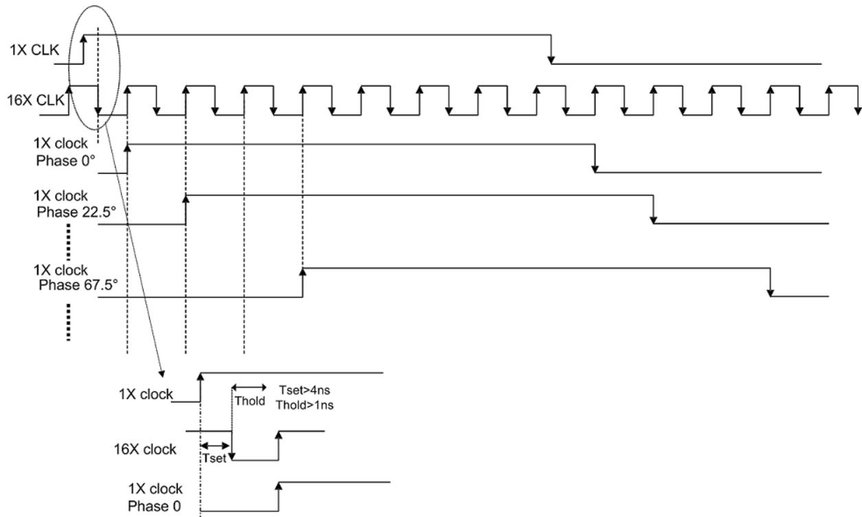
**Figure 90. 1X and 16X CW Clock Timing Diagram**
