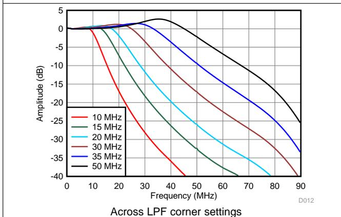
Figure 12. Full-Channel Amplitude Response vs Frequency
