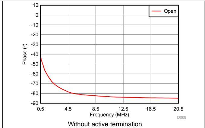
Figure 9. Input Impedance Phase vs Frequency
