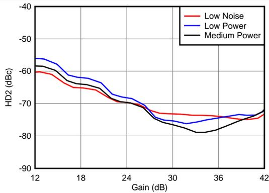
LNA = 18 dB,  $V_{OUT} = -1\text{ dBFS}$  across power modes
