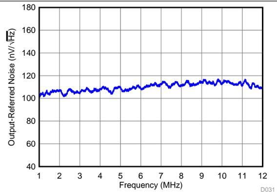
Figure 31. Output-Referred Noise vs Frequency
