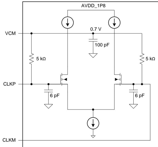
**Figure 71. Internal Clock Buffer for Differential Clock Mode**
