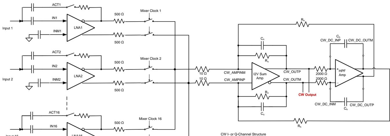
Figure 94. CW Summing Amplifier and High-Pass Filter Implementation
