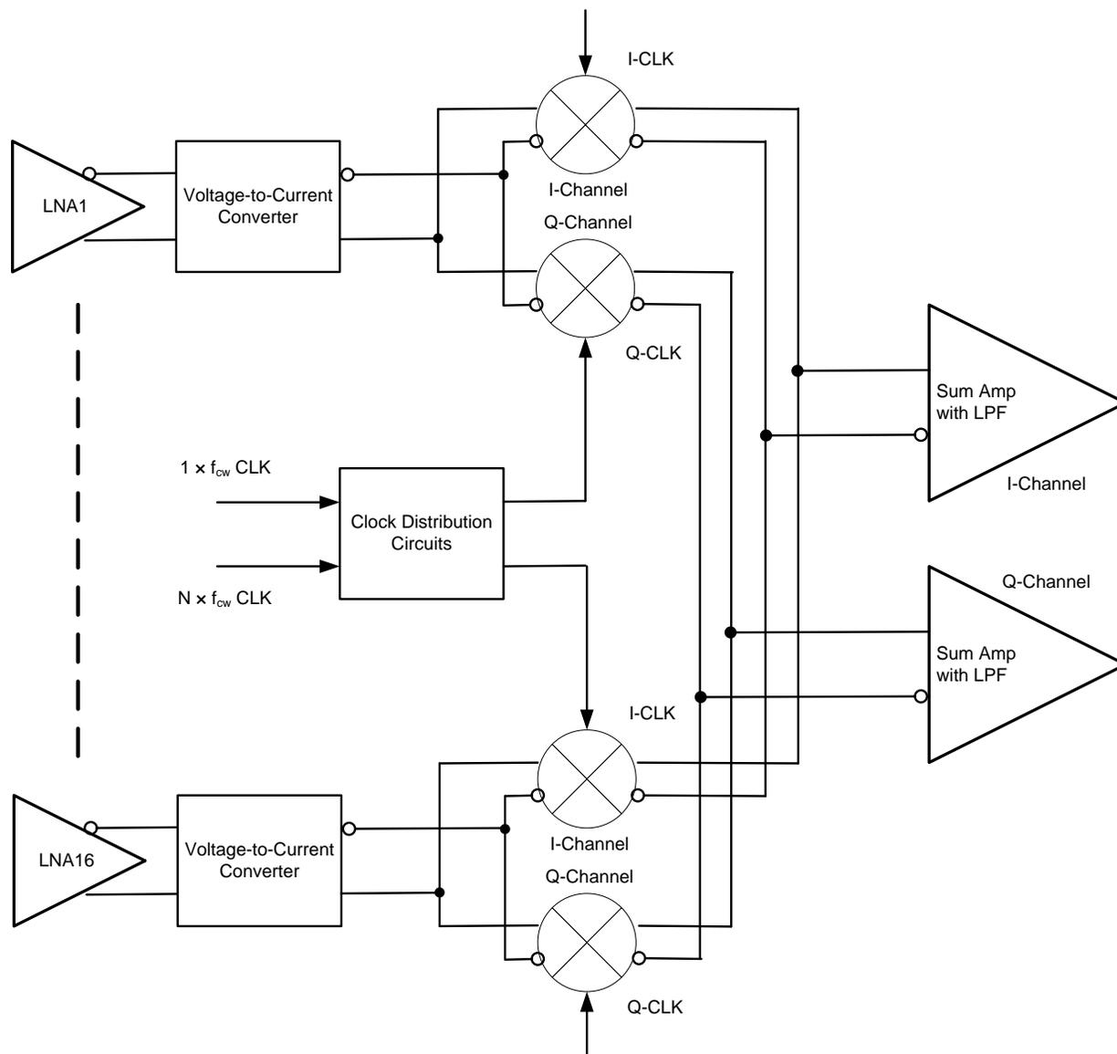
Figure 86. Simplified Block Diagram of the CW Path
