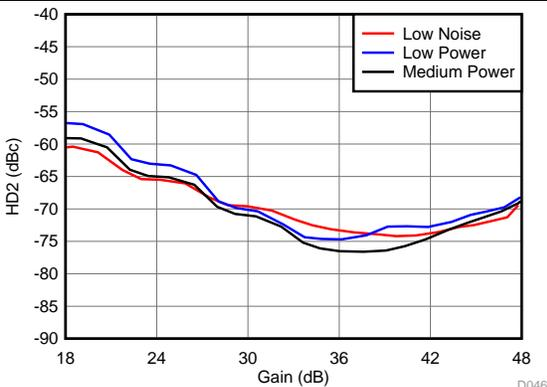
LNA = 24 dB,  $V_{OUT} = -1\text{ dBFS}$  across power modes
