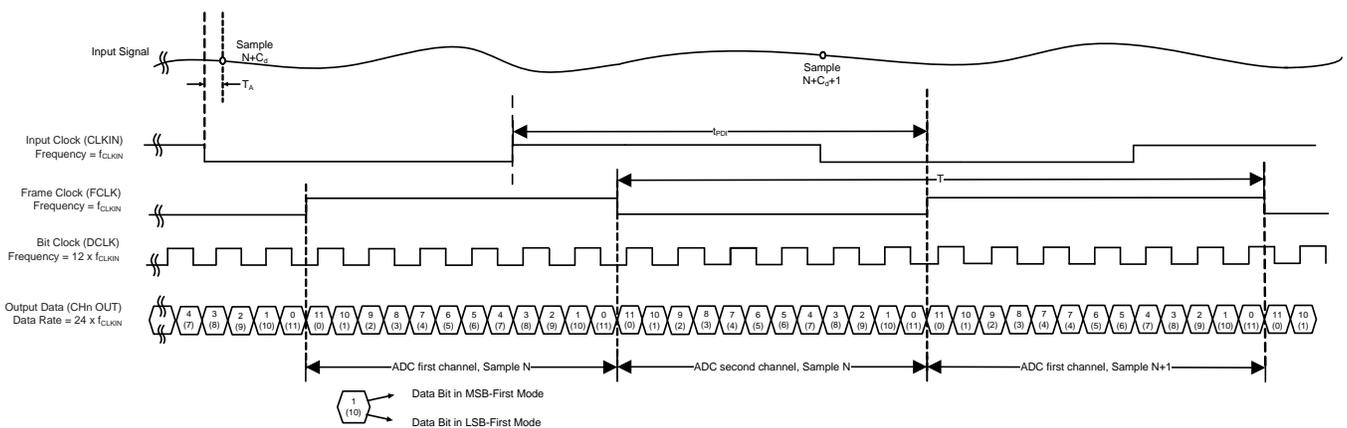
**Figure 81. 12-Bit, 2X Data Rate Output Timing Specification**
