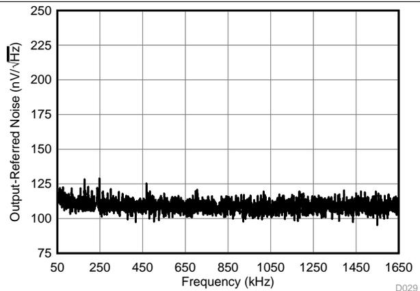
INMx capacitor =  $1\text{ }\mu\text{F}$ , PGA\_HPFF\_DIS (register 195, bit 4) = 1
