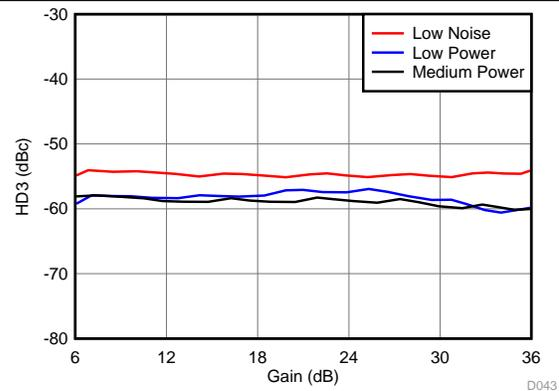
$LNA = 12\text{ dB}$ ,  $V_{OUT} = -1\text{ dBFS}$  across power modes
