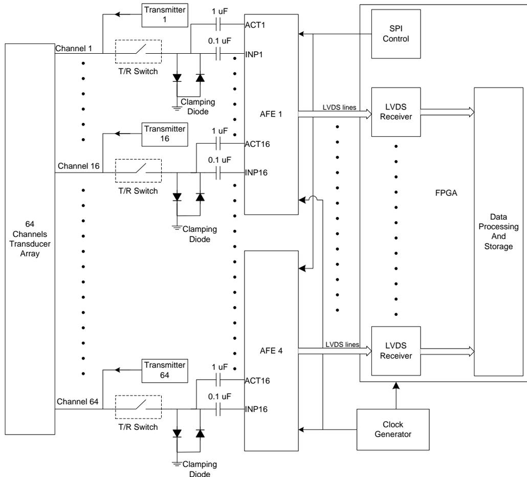
Figure 103. Simplified Schematic
