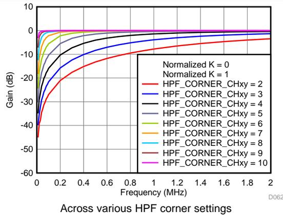
**Figure 62. Digital High-Pass Filter Gain Response vs Frequency**
