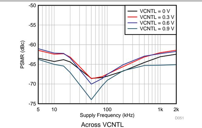
Figure 51. AVDD\_5V Power-Supply Modulation Ratio vs 100-mV<sub>pp</sub> Supply Noise Frequencies
