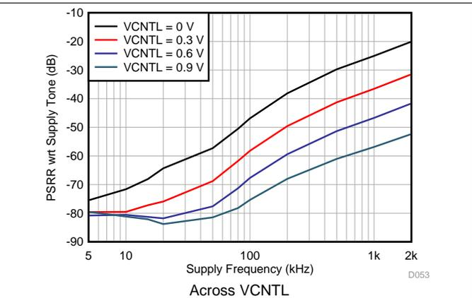
Figure 53. AVDD\_5V Power-Supply Rejection Ratio vs 100-mV<sub>pp</sub> Supply Noise Frequencies
