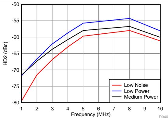
$V_{IN} = 500\text{ mV}_{PP}$ ,  $V_{OUT} = -1\text{ dBFS}$  across power modes
