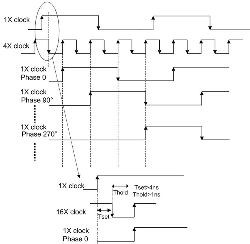
Figure 92.  $8 \times f_{cw}$  and  $4 \times f_{cw}$  Timing Diagram
