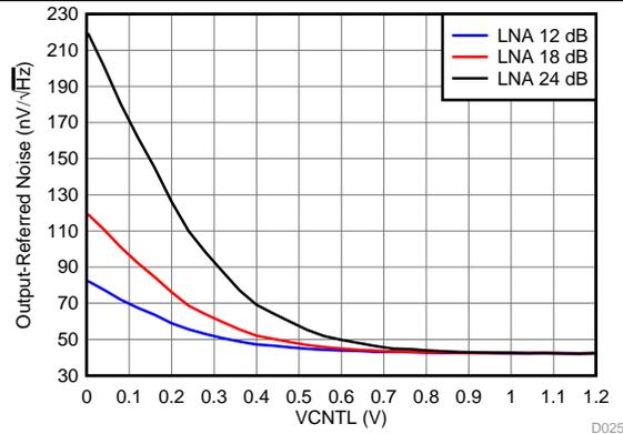
Figure 25. Output-Referred Noise vs VCNTL
