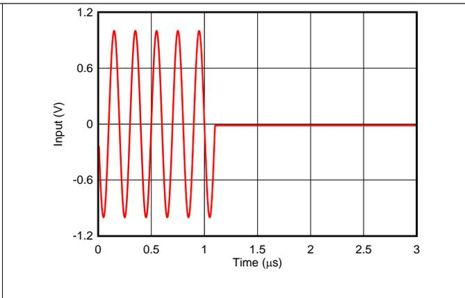
Figure 57. Pulse Inversion Asymmetrical Negative Input
