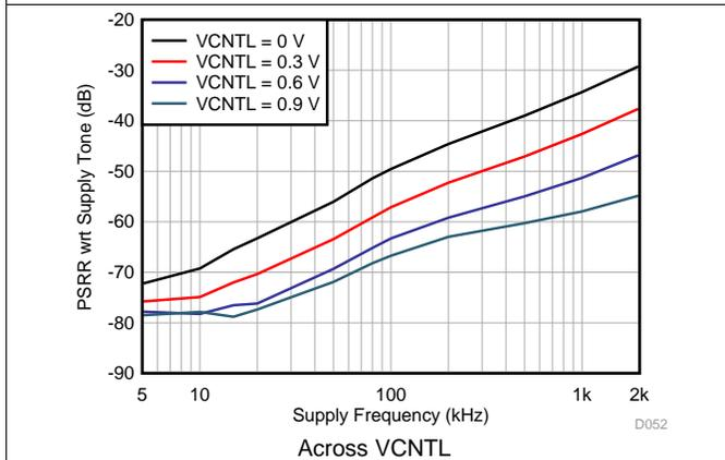
Figure 52. AVDD Power-Supply Rejection Ratio vs 100-mV<sub>pp</sub> Supply Noise Frequencies
