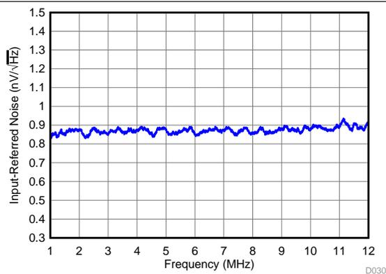
Figure 30. Input-Referred Noise vs Frequency
