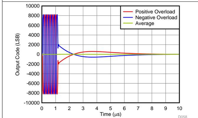
$V_{IN} = 2 V_{PP}$ , PRF = 1 kHz, gain = 21 dB, across pulse inversion asymmetrical positive and negative input
