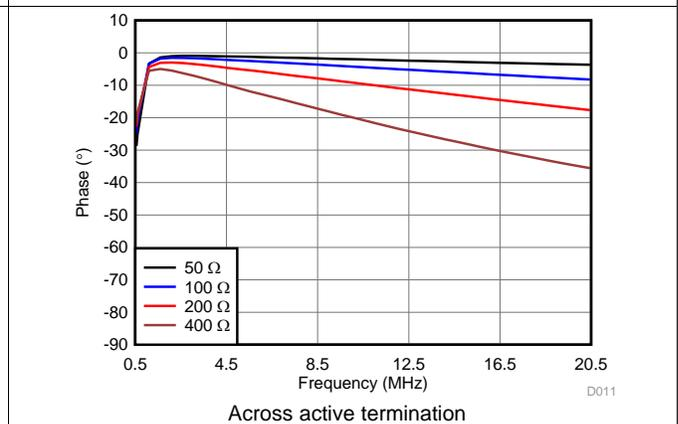
Figure 11. Input Impedance Phase vs Frequency
