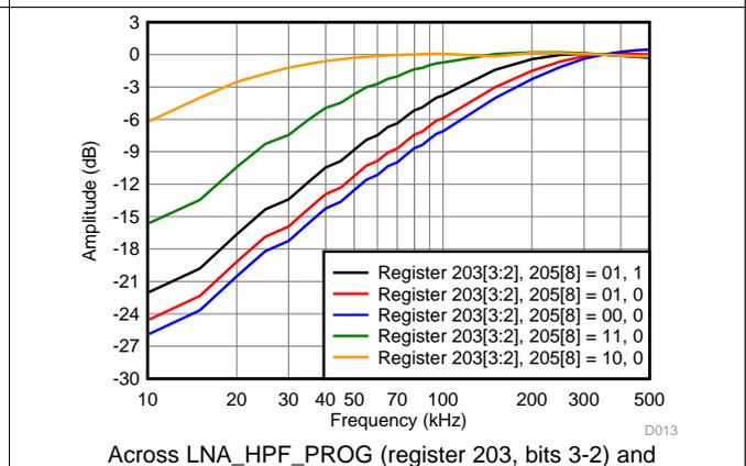
Figure 13. LNA High-Pass Filter Amplitude Response vs Frequency
