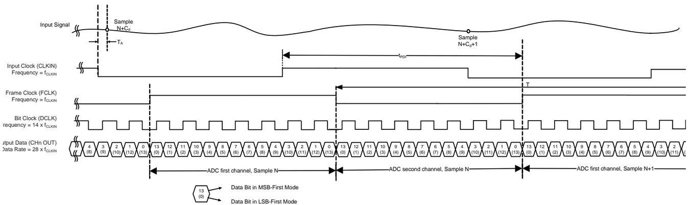
**Figure 80. 14-Bit, 2X Data Rate Output Timing Specification**
