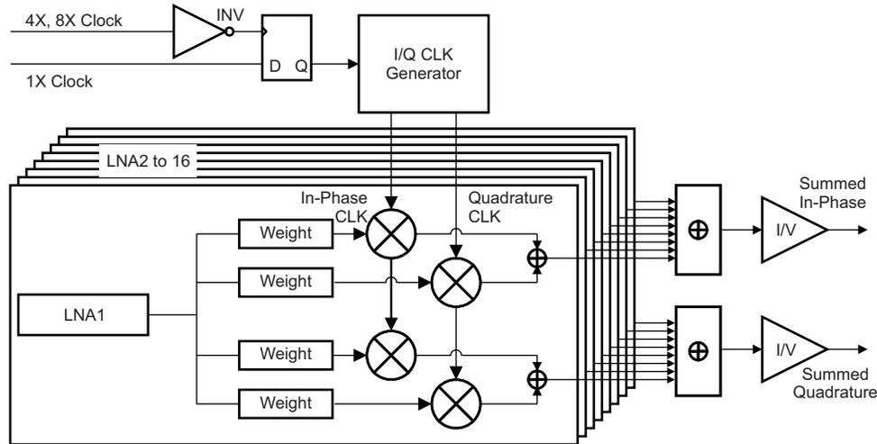
Figure 91.  $8 \times f_{CW}$  and  $4 \times f_{CW}$  Block Diagram
