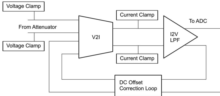
**Figure 70. Simplified Block Diagram of the PGA**
