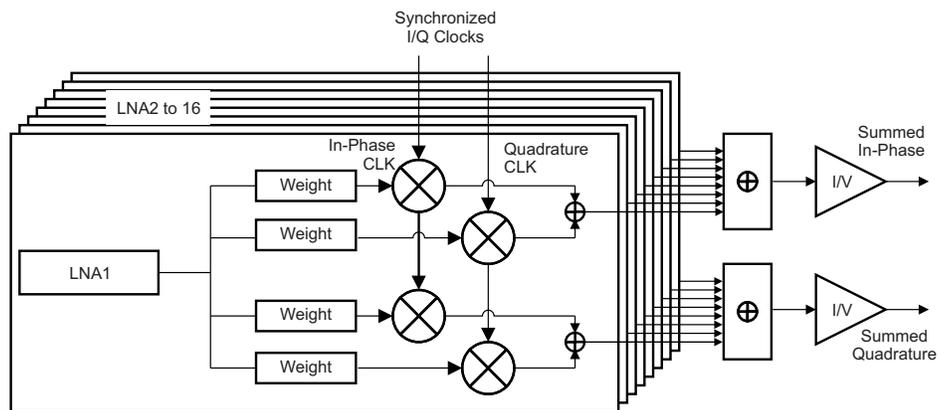
Figure 93.  $1 \times f_{cw}$  Mode Block Diagram
