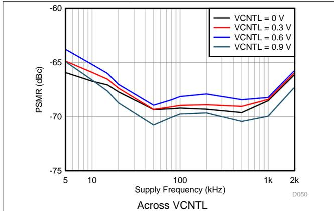
Figure 50. AVDD Power-Supply Modulation Ratio vs 100-mV<sub>pp</sub> Supply Noise Frequencies
