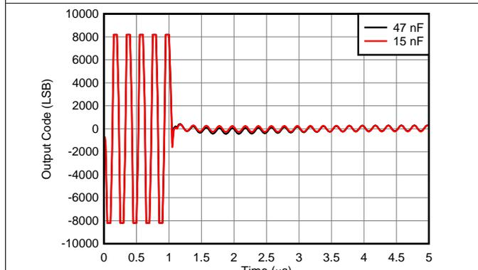
$V_{IN} = \text{large amplitude (50 mV}_{PP})$  followed by small amplitude ( $500\text{ }\mu\text{V}_{PP}$ ), across INM capacitor
