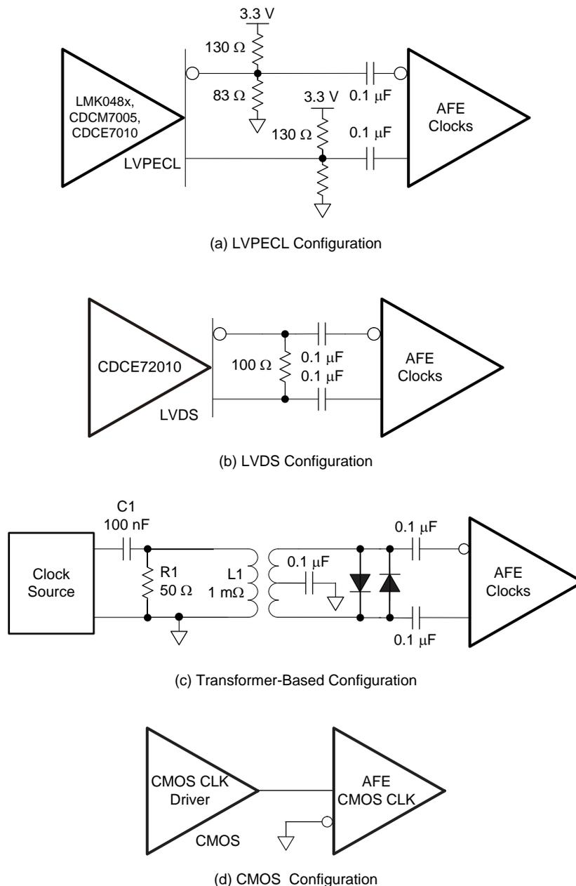
**Figure 97. Clock Configurations**
