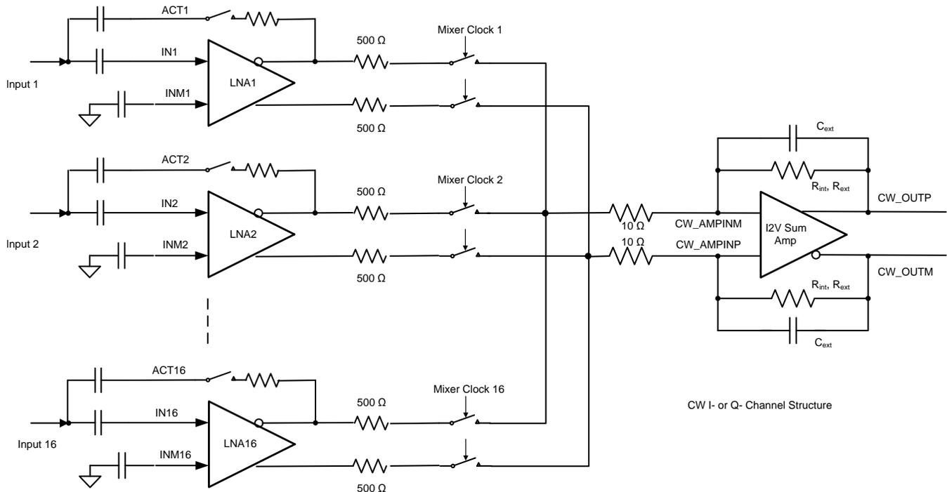
NOTE: The 10-Ω to 15-Ω resistors at CW\_AMPINM and CW\_AMPINP result from the internal device routing and can create slight attenuation.
