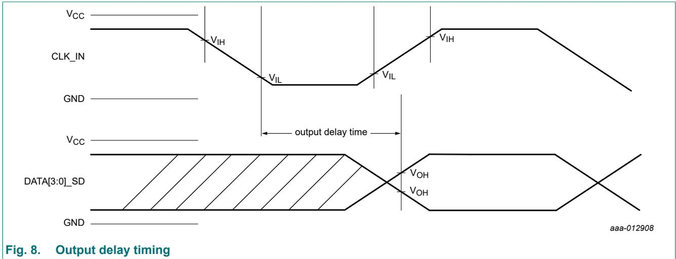
Fig. 8. Output delay timing
