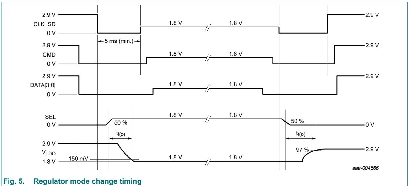
Fig. 5. Regulator mode change timing
