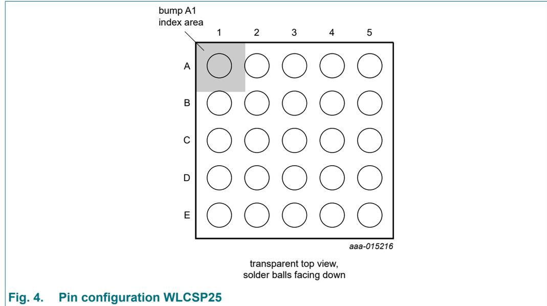
Fig. 4. Pin configuration WLCSP25
