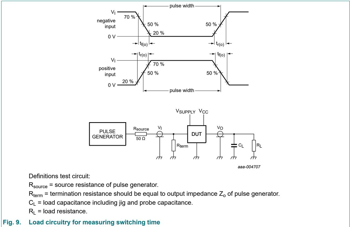
Fig. 9. Load circuitry for measuring switching time
