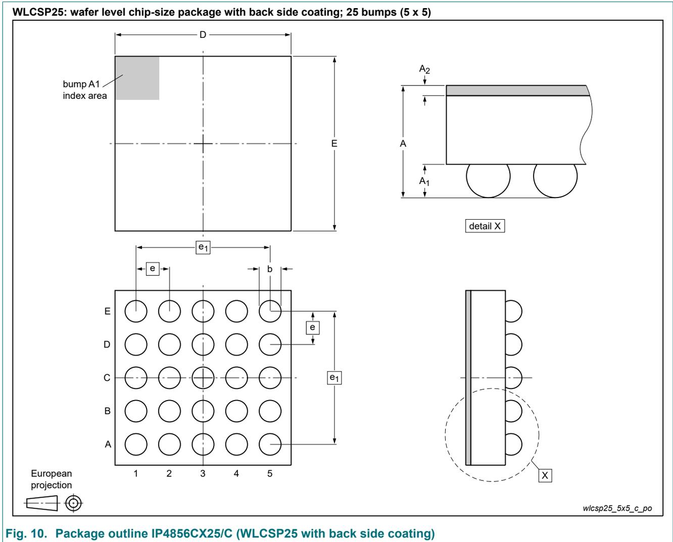
Fig. 10. Package outline IP4856CX25/C (WLCSP25 with back side coating)
