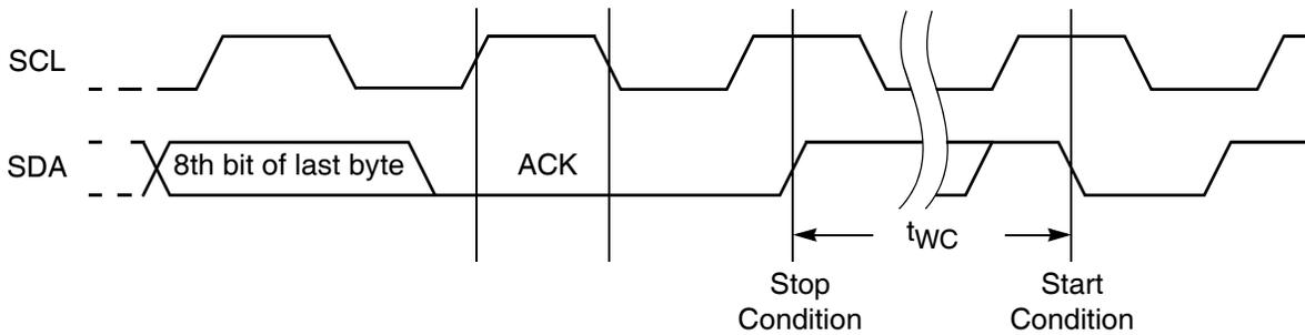
Figure 25. DCP “Wiper Position” Timing
