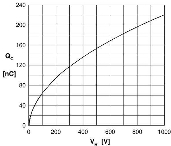
Fig. 5 Typ. recovery charge vs. reverse voltage
