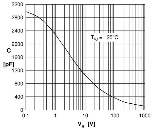
Fig. 6 Typ. junction capacitance vs. reverse Voltage
