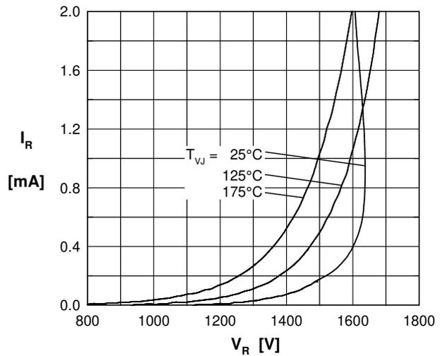
Fig. 2 Typ. reverse characteristics
