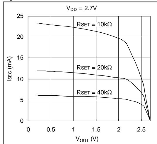
Figure 9.  $I_{SEG}$  vs.  $R_{SET}$
