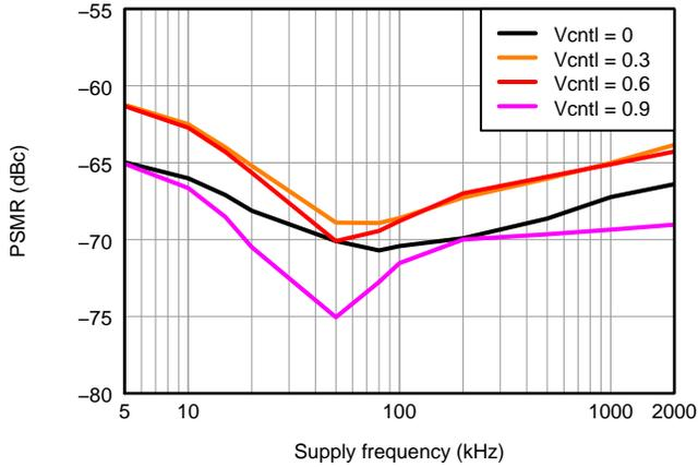
**Figure 48. AVDD 5V Power Supply Modulation Ratio, 100 mV<sub>PP</sub> Supply Noise With Different Frequencies**
