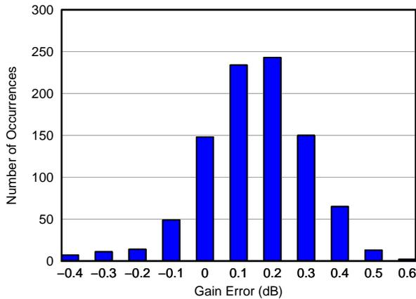
Figure 4. Gain Matching Histogram, VCNTL = 0.3 V (936 channels)
