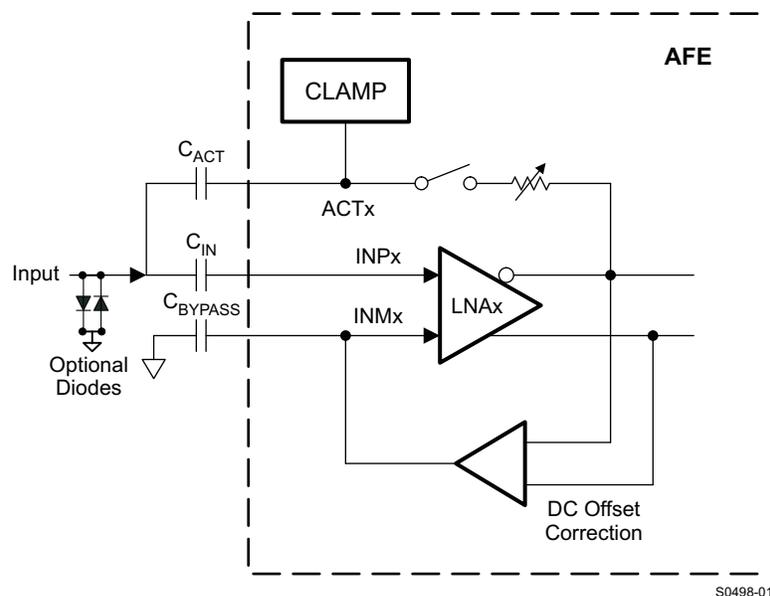
Figure 64. AFE5808 LNA With DC Offset Correction Circuit
