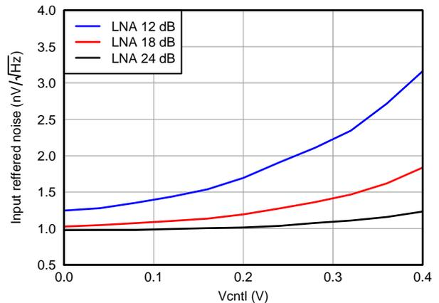
Figure 21. IRN, PGA = 24 dB and Medium Power Mode
