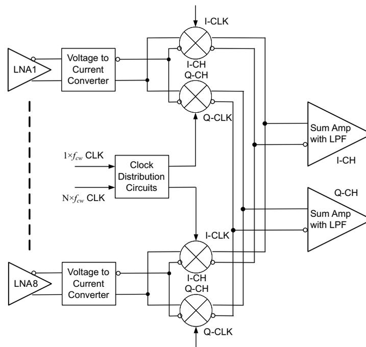
Figure 68. Simplified Block Diagram of CW Path
