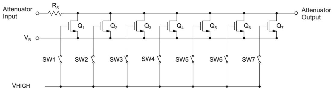
Figure 66. Simplified Voltage Controlled Attenuator (Digital Structure)
