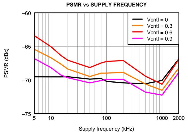
Figure 47. AVDD Power Supply Modulation Ratio, 100 mV<sub>PP</sub> Supply Noise With Different Frequencies
