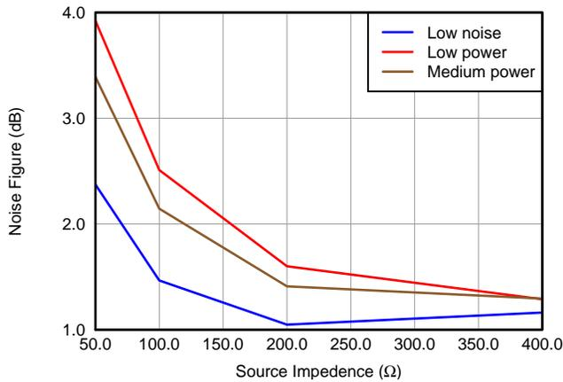
**Figure 36. Noise Figure vs Power Modes Without Termination**
