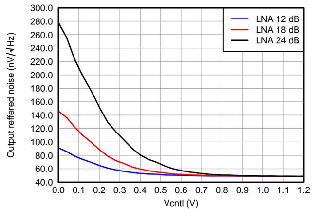
Figure 25. ORN, PGA = 24 dB and Medium Power Mode
