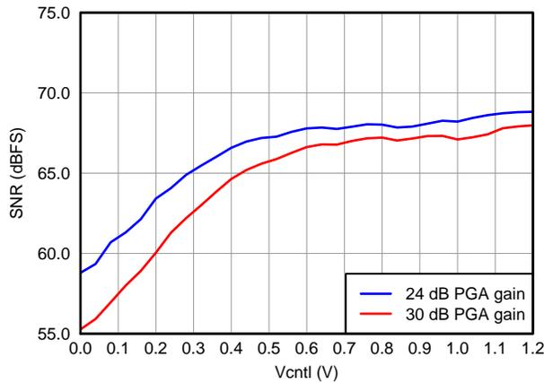
Figure 30. SNR, LNA = 18 dB and Low Power Mode
