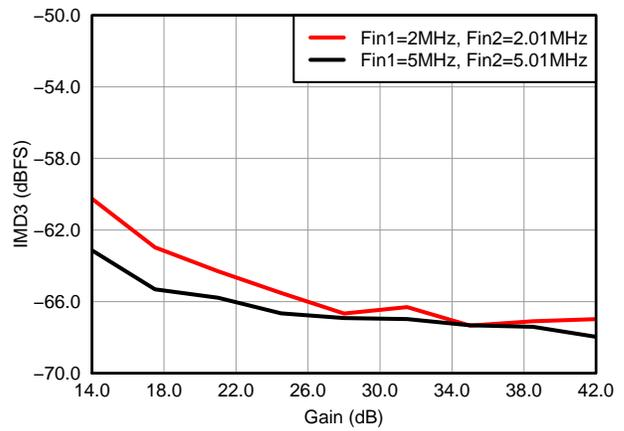
Figure 45. IMD3,  $F_{out1} = -7$  dBFS and  $F_{out2} = -21$  dBFS
