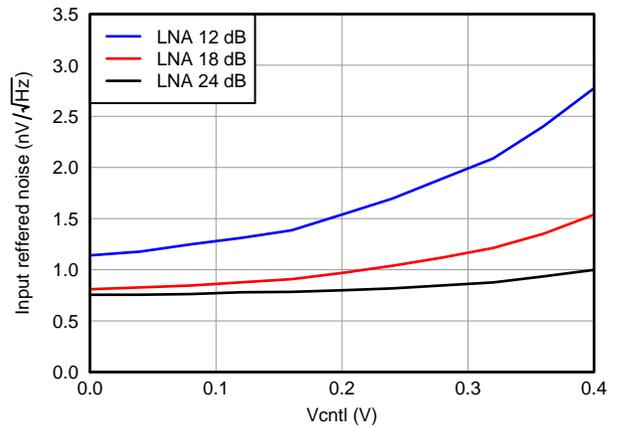
Figure 19. IRN, PGA = 24 dB and Low Noise Mode
