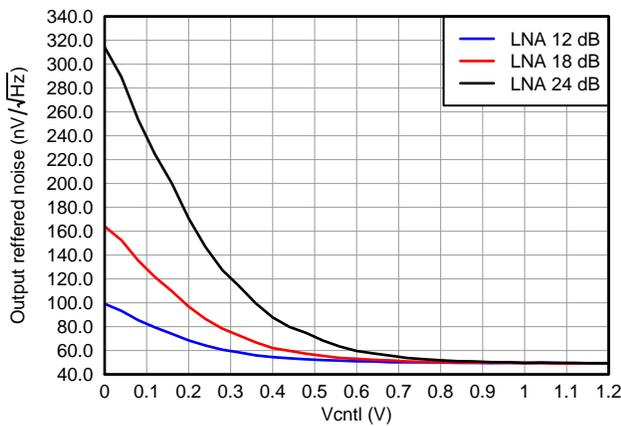
Figure 26. ORN, PGA = 24 dB and Low Power Mode
