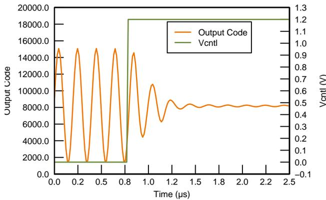
**Figure 52. V<sub>CNTL</sub> Response Time, LNA = 18 dB and PGA = 24 dB**
