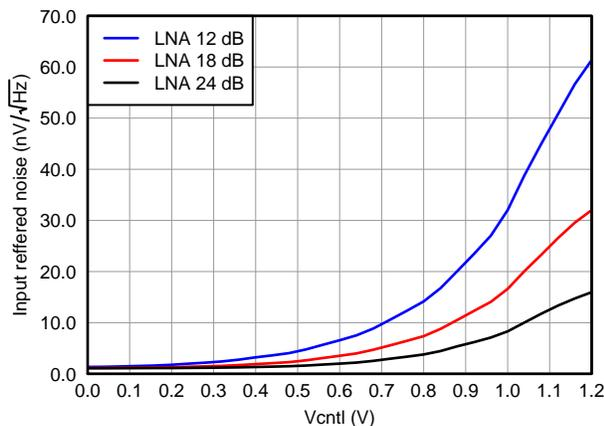
Figure 22. IRN, PGA = 24 dB and Low Power Mode
