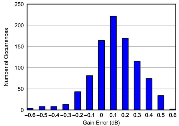
Figure 5. Gain Matching Histogram, VCNTL = 0.6 V (936 channels)
