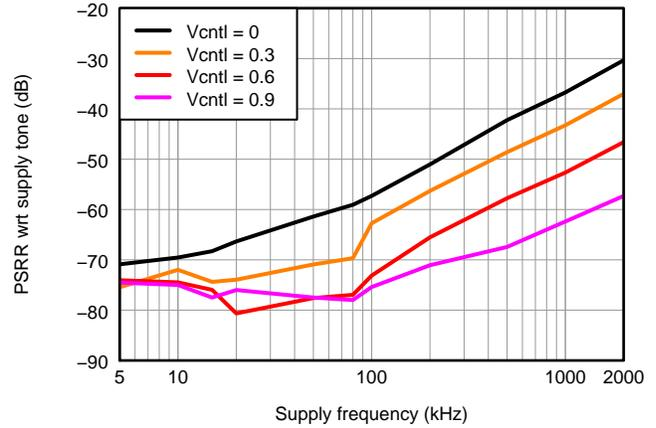
**Figure 49. AVDD Power Supply Rejection Ratio, 100 mV<sub>PP</sub> Supply Noise With Different Frequencies**
