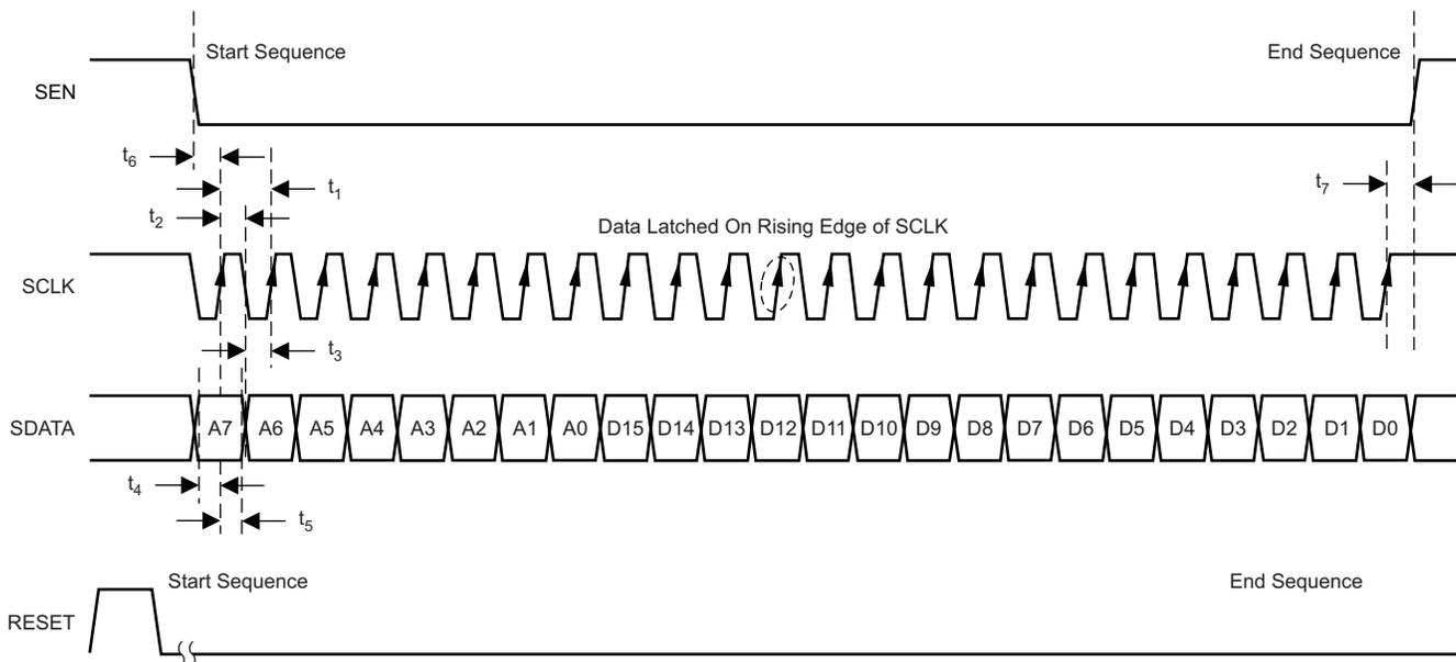
**Figure 59. SPI Timing**
