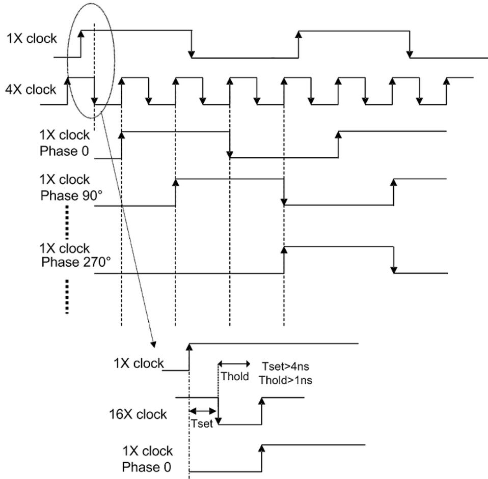
Figure 74.  $8 \times f_{cw}$  and  $4 \times f_{cw}$  Timing Diagram
