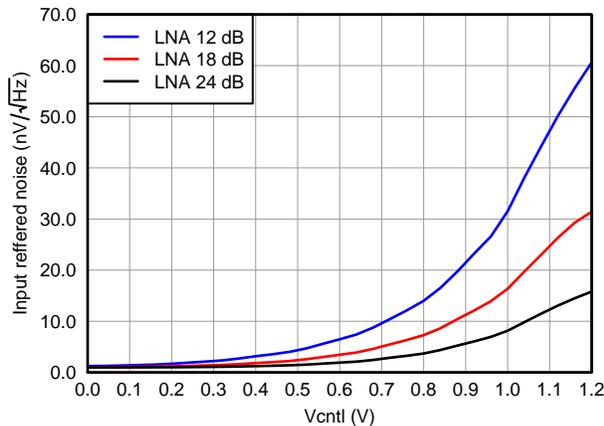
Figure 20. IRN, PGA = 24 dB and Medium Power Mode
