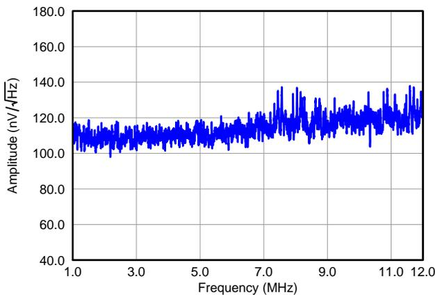
Figure 28. ORN, PGA = 24 dB and Low Noise Mode
