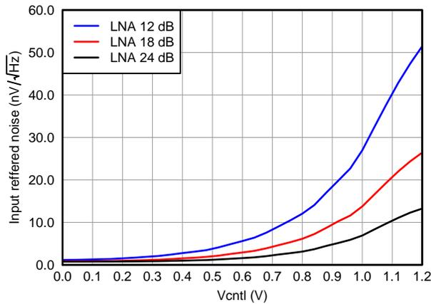
Figure 18. IRN, PGA = 24 dB and Low Noise Mode
