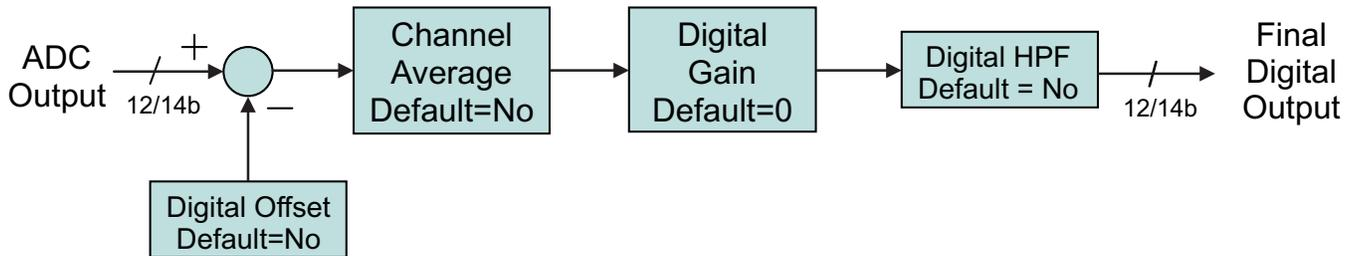
Figure 62. ADC Digital Block Diagram
