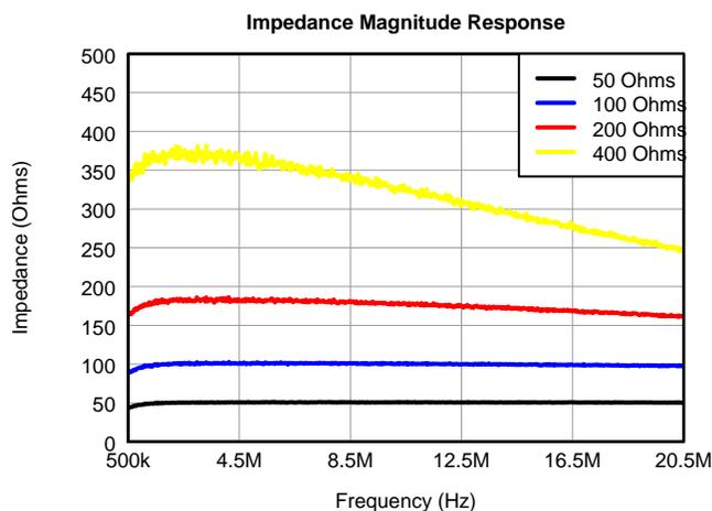
Figure 10. Input Impedance With Active Termination (Magnitude)
