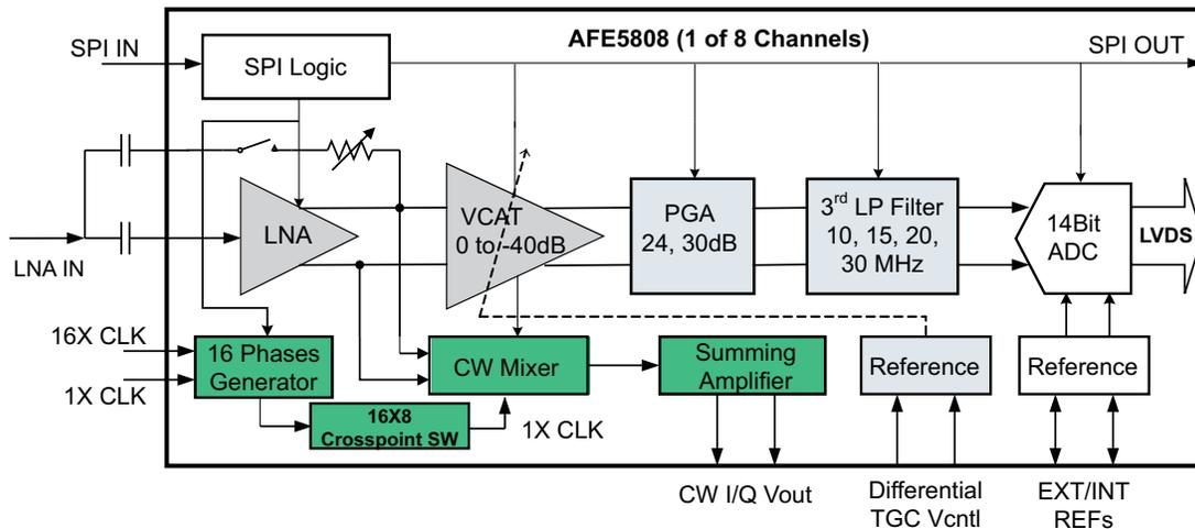
Figure 1. Block Diagram
