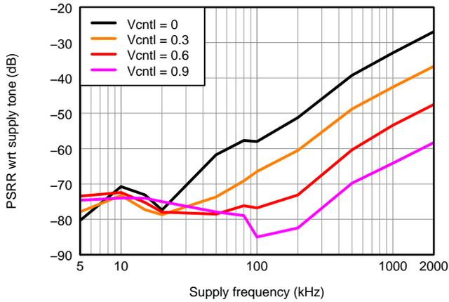
**Figure 50. AVDD 5V Power Supply Rejection Ratio, 100 mV<sub>PP</sub> Supply Noise With Different Frequencies**
