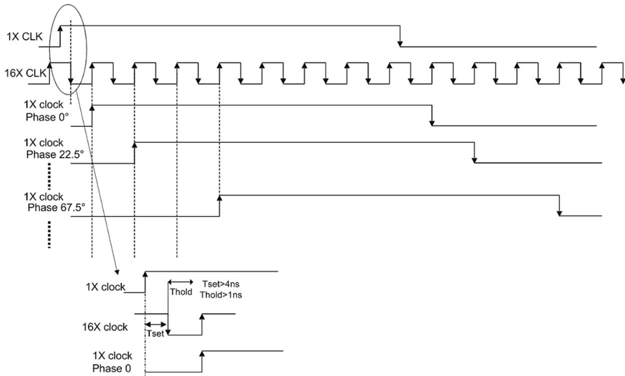
Figure 72. 1x and 16x CW Clock Timing
