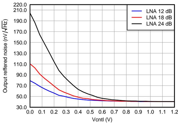
Figure 24. ORN, PGA = 24 dB and Low Noise Mode
