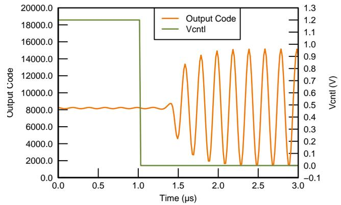
**Figure 51. V<sub>CNTL</sub> Response Time, LNA = 18 dB and PGA = 24 dB**
