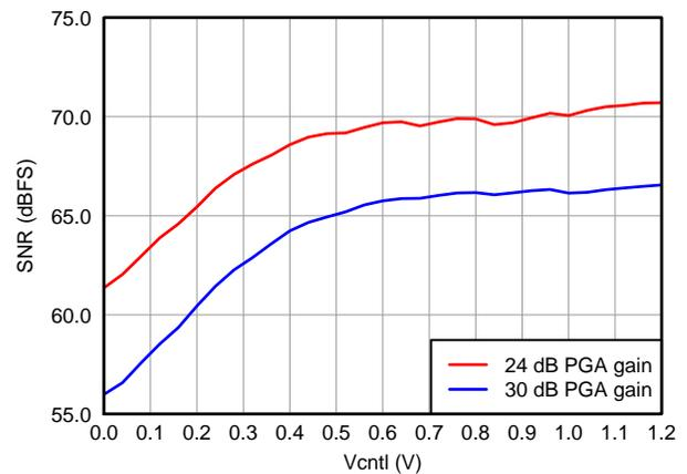
Figure 29. SNR, LNA = 18 dB and Low Noise Mode
