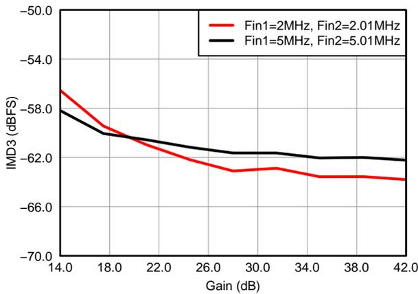
Figure 46. IMD3,  $F_{out1} = -7$  dBFS and  $F_{out2} = -7$  dBFS
