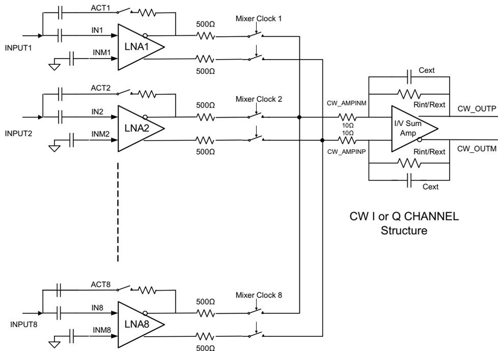
Note: the 10~15Ω resistors at CW\_AMPINM/P are due to internal IC routing and can create slight attenuation.
