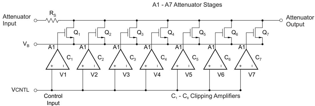
Figure 65. Simplified Voltage Controlled Attenuator (Analog Structure)
