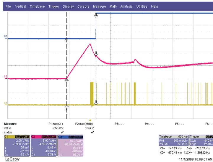
Figure 6. Start-Up Sequence Waveforms (Ch1 (Y), PFCDRV, Ch2 (R), V<sub>CCA</sub>, Ch3 (B), DUT V<sub>O</sub>)
