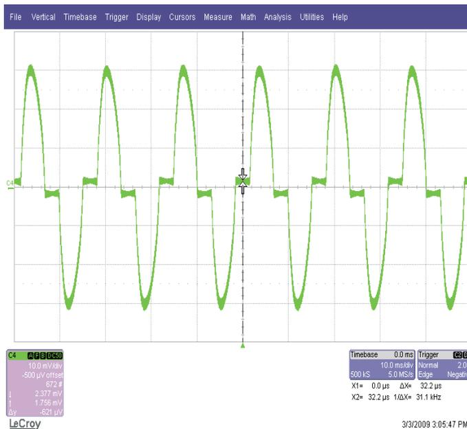
Figure 3. 115 V, 60 Hz, Full Load, 0.5 A/div
