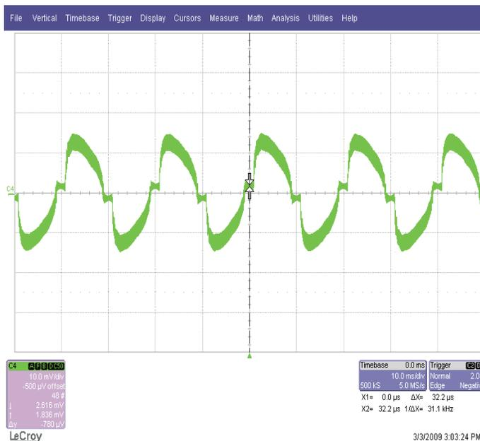
Figure 4. 230 V, 50 Hz, Full Load, 0.5 A/div
