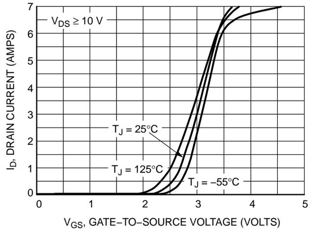
**Figure 2. Transfer Characteristics**
