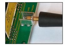
SCRTM4RA is a PCB Mounting terminal which accept any M4 screw thread antenna. For further data please see DS-SCRTM4RA
