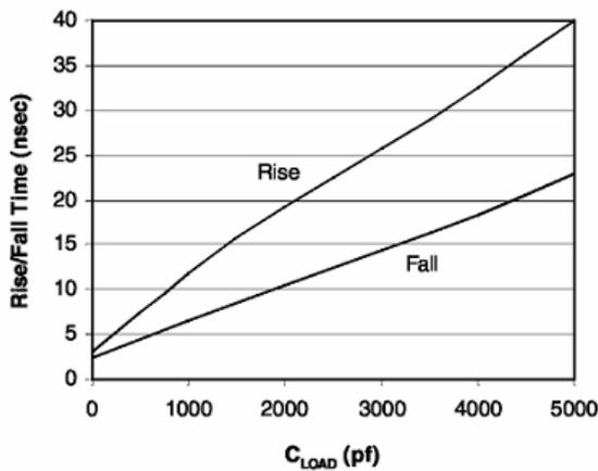
Figure 9. HDRV Rise and Fall Times vs. C<sub>LOAD</sub>
