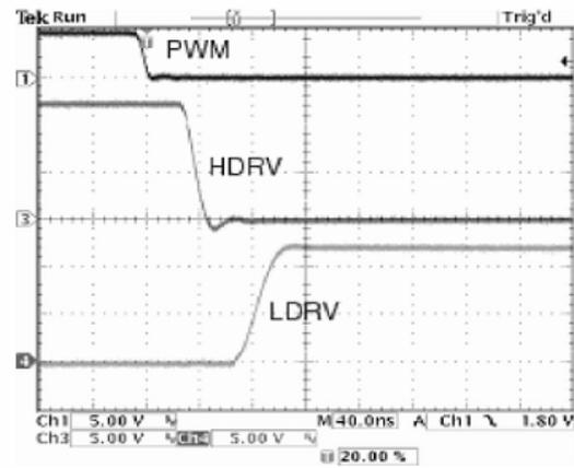
Figure 8. Gate Drive Rise and Fall Times (2)
