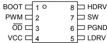
Figure 3. Pin Assignments
