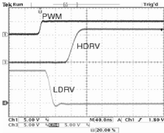
Figure 7. Gate Drive Rise and Fall Times (1)
