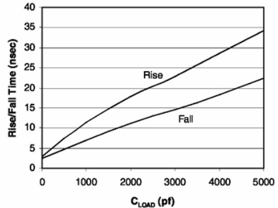
Figure 10. LDRV Rise and Fall Times vs. C<sub>LOAD</sub>
