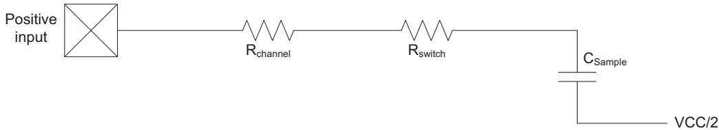
**Figure 25-19. ADC Input for Differential Measurements and Differential Measurements with Gain**
