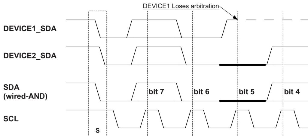
Figure 19-9 shows an example where two TWI masters are contending for bus ownership. Both devices are able to issue a START condition, but DEVICE1 loses arbitration when attempting to transmit a high level (bit 5) while DEVICE2 is transmitting a low level.
