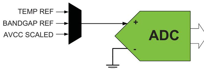
To measure the internal signals in unsigned mode, the negative input is connected to a fixed value given by the formula below, which is half of the voltage reference (VREF) minus a fixed offset, as it is for single-ended unsigned input. Refer to [Figure 25-11 on page 285](#) for details.
