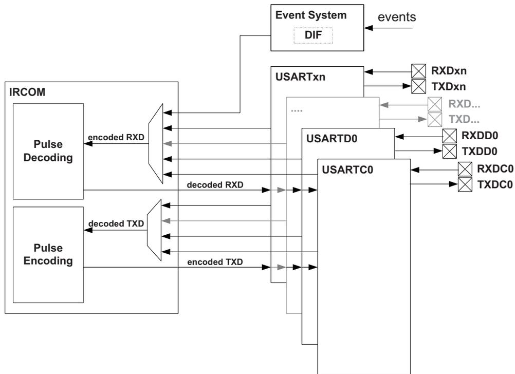
The IRCOM is automatically enabled when a USART is set in IRCOM mode. The signals between the USART and the RX/TX pins are then routed through the module as shown in Figure 22-1. The data on the TX/RX pins are the inverted value of the transmitted/received infrared pulse. It is also possible to select an event channel from the event system as input for the IRCOM receiver. This will disable the RX input from the USART pin.
