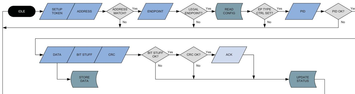
The USB module then fetches the endpoint data pointer register (DATAPTR) and waits for a DATA0 packet. If a PID error or any other PID than DATA0 is detected, the USB module returns to idle and waits for the next token packet.
