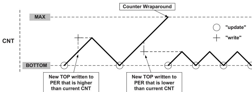
When double buffering is used, the buffer can be written at any time and still maintain correct operation. The period register is always updated on the UPDATE condition, as shown for dual-slope operation in [Figure 13-9 on page 148](#). This prevents wraparound and the generation of odd waveforms.
