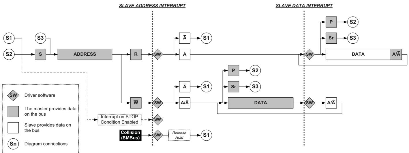
The number of interrupts generated is kept to a minimum by automatic handling of most conditions. Quick command can be enabled to auto-trigger operations and reduce software complexity.
