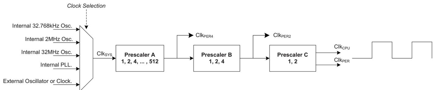
Prescaler A divides the system clock, and the resulting clock is  $clk_{PER4}$ . Prescalers B and C can be enabled to divide the clock speed further to enable peripheral modules to run at twice or four times the CPU clock frequency. If Prescalers B and C are not used, all the clocks will run at the same frequency as the output from Prescaler A.
