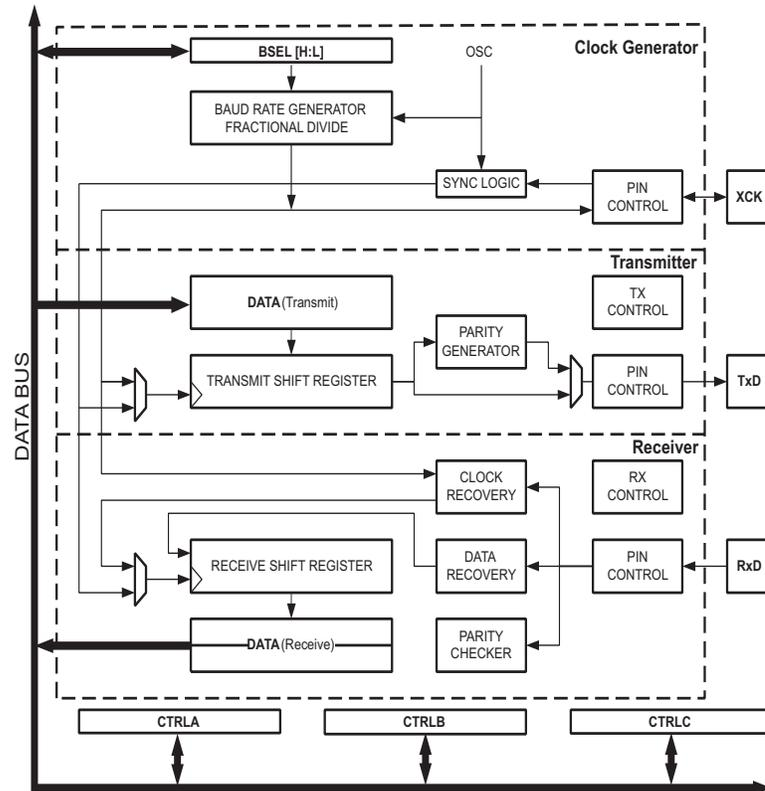
The clock generator includes a fractional baud rate generator that is able to generate a wide range of USART baud rates from any system clock frequencies. This removes the need to use an external crystal oscillator with a specific frequency to achieve a required baud rate. It also supports external clock input in synchronous slave operation.
