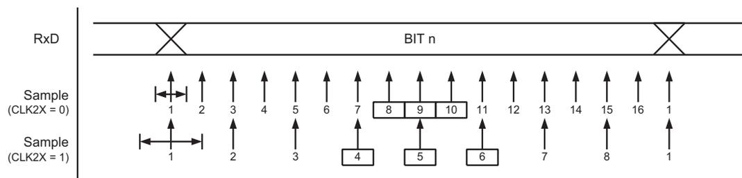
As for start bit detection, an identical majority voting technique is used on the three center samples for deciding of the logic level of the received bit. The process is repeated for each bit until a complete frame is received. It includes the first stop bit, but excludes additional ones. If the sampled stop bit is a 0 value, the frame error (FERR) flag will be set.
