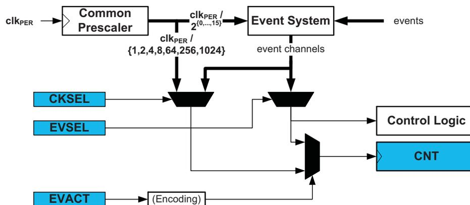
The peripheral clock is fed into a common prescaler (common for all timer/counters in a device). Prescaler outputs from 1 to 1/1024 are directly available for selection by the timer/counter. In addition, the whole range of prescaling from 1 to 2<sup>15</sup> times is available through the event system.
