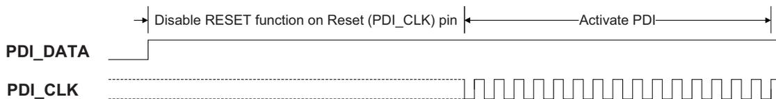
The Reset pin is sampled when the PDI interface is enabled. The reset register is then set according to the state of the Reset pin, preventing the device from running code after the reset functionality of this pin is disabled.
