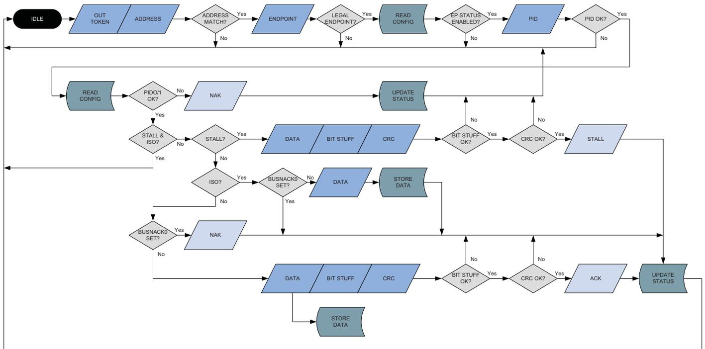
The USB module then fetches the endpoint DATAPTR register and waits for a DATA0 or DATA1 packet. If a PID error or any other PID than DATA0 or DATA1 is detected, the USB module returns to idle and waits for the next token packet.
