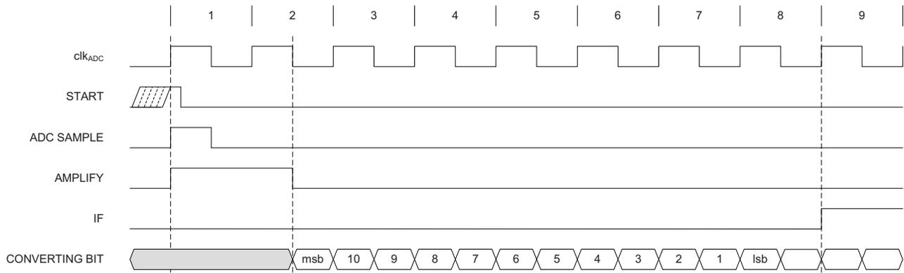
**Figure 25-17. ADC Timing for One Single Conversion with 64x Gain**
