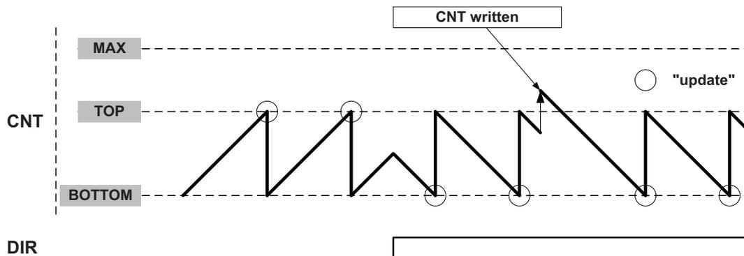
As shown in [Figure 13-6](#), it is possible to change the counter value when the counter is running. The write access has higher priority than count, clear, or reload, and will be immediate. The direction of the counter can also be changed during normal operation.
