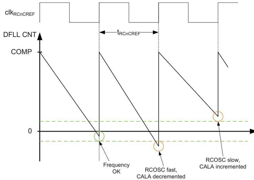
The DFLF will stop when entering a sleep mode where the oscillators are stopped. After wake up, the DFLF will continue with the calibration value found before entering sleep. The reset value of the DFLF calibration register can be read from the production signature row.
