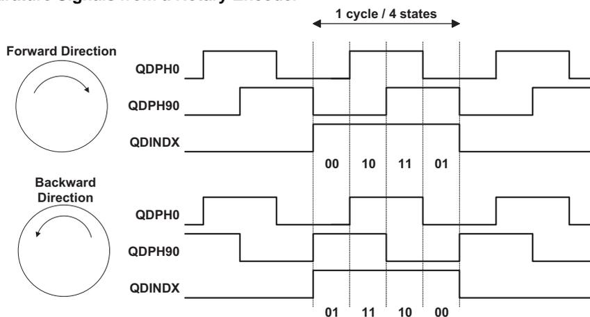
[Figure 6-4](#) shows typical quadrature signals from a rotary encoder. The signals QDPH0 and QDPH90 are the two quadrature signals. When QDPH90 leads QDPH0, the rotation is defined as positive or forward. When QDPH0 leads QDPH90, the rotation is defined as negative or reverse. The concatenation of the two phase signals is called the quadrature state or the phase state.
