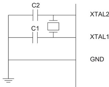
Two capacitors, C1 and C2, may be added to match the required load capacitance for the connected crystal.
