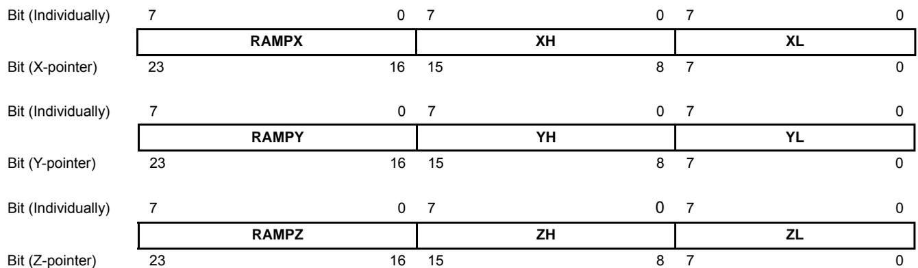
When reading (ELPM) and writing (SPM) program memory locations above the first 128KB of the program memory, RAMPZ is concatenated with the Z-register to form the 24-bit address. LPM is not affected by the RAMPZ setting.
