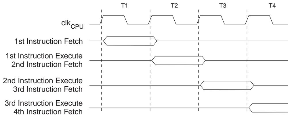
Figure 3-3 shows the internal timing concept for the register file. In a single clock cycle, an ALU operation using two register operands is executed and the result is stored back to the destination register.
