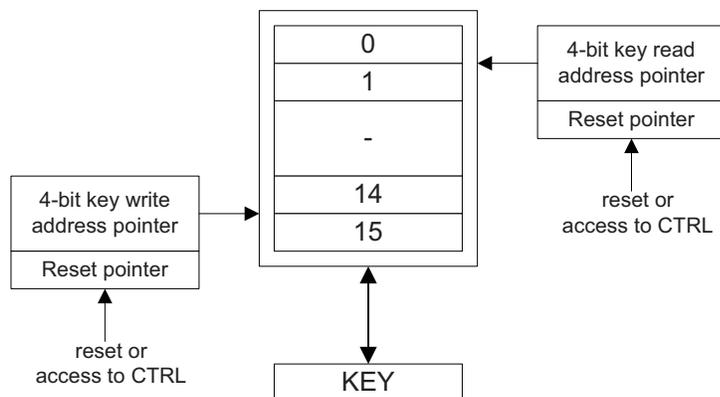
In the AES crypto module, the following definition of the key is used:
