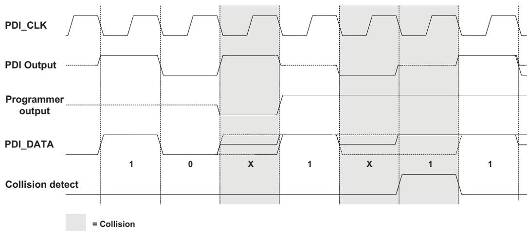
As long as the PDI transmits alternating ones and zeros, collisions cannot be detected, because the PDI output driver will be active all the time, preventing polling of the PDI\_DATA line. However, the two stop bits should always be transmitted as ones within a single frame, enabling collision detection at least once per frame.
