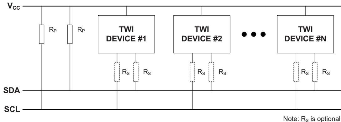
A unique address is assigned to all slave devices connected to the bus, and the master will use this to address a slave and initiate a data transaction.
