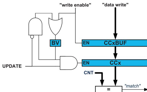
When the CC channels are used for a capture operation, a similar double buffering mechanism is used, but in this case the buffer valid flag is set on the capture event, as shown in Figure 13-5 on page 146. For capture, the buffer register and
