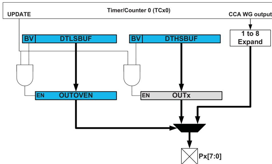
As with the other timer/counter double buffered registers, the register update is synchronized to the UPDATE condition set by the waveform generation mode. If the synchronization provided is not required by the application, the application code can simply access the DTIOE and PORTx registers directly.
