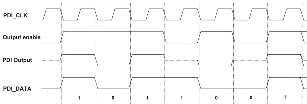
If the programmer and the PDI both drive the PDI\_DATA line at the same time, drive contention will occur, as illustrated in Figure 27-9. Every time a bit value is kept for two or more clock cycles, the PDI is able to verify that the correct bit value is driven on the PDI\_DATA line. If the programmer is driving the PDI\_DATA line to the opposite bit value to what the PDI expects, a collision is detected.
