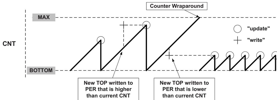
A counter wraparound can occur in any mode of operation when up-counting without buffering, as shown in [Figure 13-8](#). This is due to the fact that CNT and PER are continuously compared, and if a new TOP value that is lower than current CNT is written to PER, it will wrap before a compare match happens.
