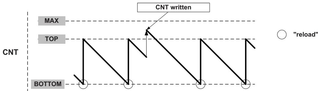
As shown in Figure 14-3, the counter can change the counter value while running. The write access has higher priority than the count clear, and reloads and will be immediate.
