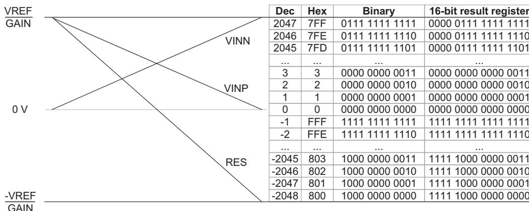
**Figure 25-10. Signed Single-ended and Internal Input, Input Range, and Result Representation**
