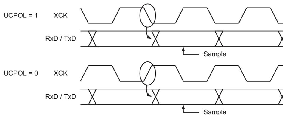
Using the inverted I/O (INVEN) setting for the corresponding XCK port pin, the XCK clock edges used for data sampling and data change can be selected. If inverted I/O is disabled (INVEN=0), data will be changed at the rising XCK clock edge and sampled at the falling XCK clock edge. If inverted I/O is enabled (INVEN=1), data will be changed at the falling XCK clock edge and sampled at the rising XCK clock edge. For more details, see “I/O Ports” on page 119.
