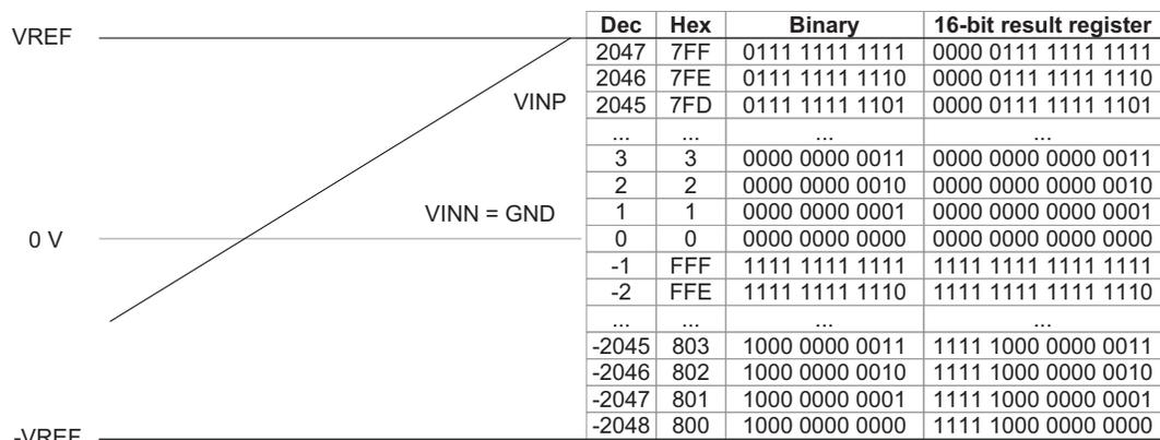
**Figure 25-11. Unsigned Single-ended and Internal Input, Input Range, and Result Representation**
