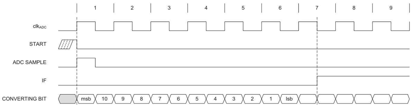
**Figure 25-14. ADC Timing for One Single Conversion with Increased Sampling Time (SAMPVAL = 6)**
