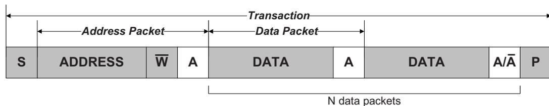
Assuming the slave acknowledges the address, the master can start transmitting data (DATA) and the slave will ACK or NACK ( $A/\overline{A}$ ) each byte. If no data packets are to be transmitted, the master terminates the transaction by issuing a STOP condition (P) directly after the address packet. There are no limitations to the number of data packets that can be
