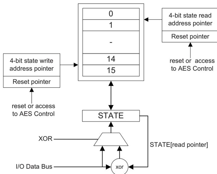
The state memory contains the AES state throughout the encryption/decryption process. The initial value of the state is the initial data (i.e., plaintext in the encryption mode, and ciphertext in the decryption mode). The last value of the state is the encrypted/decrypted data.
