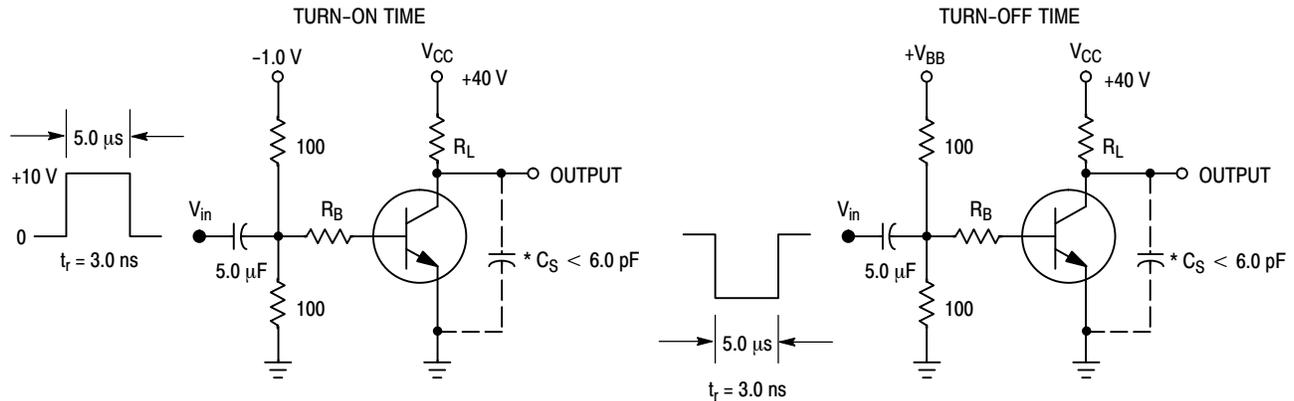
\*Total Shunt Capacitance of Test Jig and Connectors
