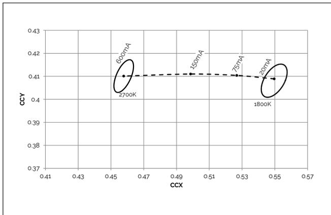
**Figure 4: Color Shift vs. Forward Current 3000K - 1800K**
