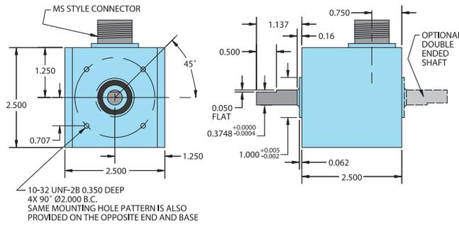
All dimensions are in inches with a tolerance of +0.005" or +0.01" unless otherwise specified
