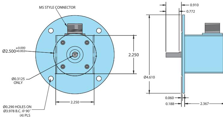
All dimensions are in inches with a tolerance of +0.005" or +0.01" unless otherwise specified.
