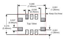
\* Do not route any traces in the keep out area. It is recommended the next layer under the keep out area is to be ground plane.
