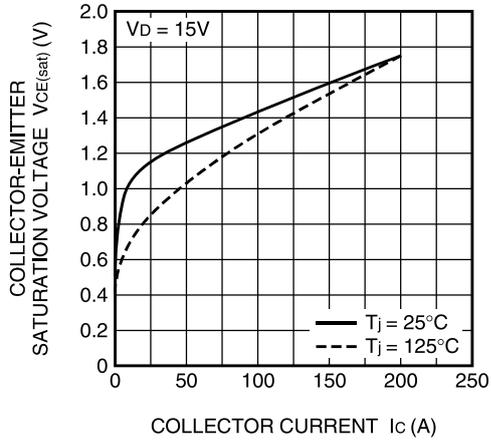
**COLLECTOR-EMITTER SATURATION VOLTAGE (VS.  $V_D$ ) CHARACTERISTICS (TYPICAL)**
