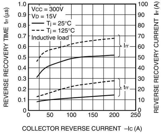
**SWITCHING RECOVERY LOSS CHARACTERISTICS (TYPICAL)**
