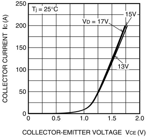
**COLLECTOR-EMITTER SATURATION VOLTAGE (VS.  $I_c$ ) CHARACTERISTICS (TYPICAL)**
