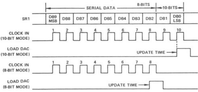
Figure 9. Timing Diagram for Serial 8- and 10-Bit Loading
