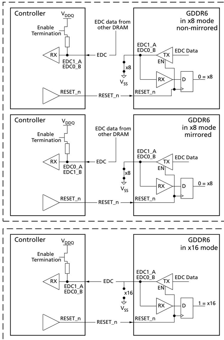
**Figure 9: System View for x16 and x8 Modes**
