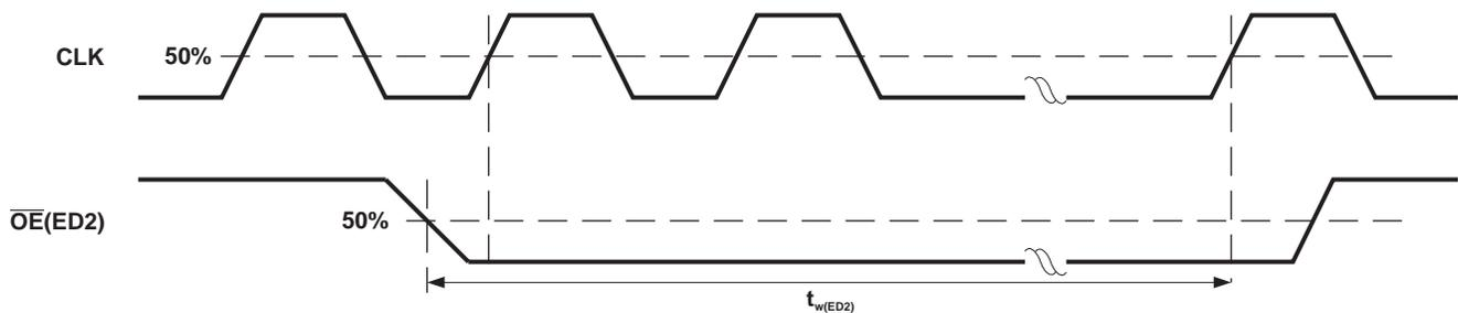
**Figure 8. Reading Error Status Code Timing Waveforms**
