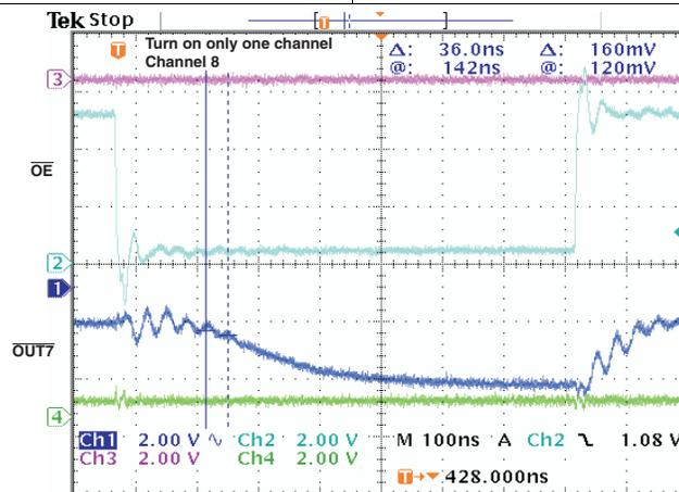
Figure 3. Response Time,  $\overline{\text{OE}}$  to  $\overline{\text{OUT7}}$
