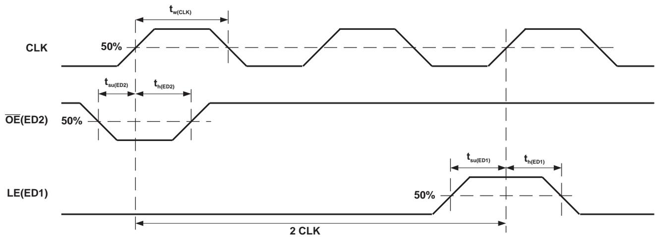
**Figure 7. Switching to Special Mode Timing Waveforms**
