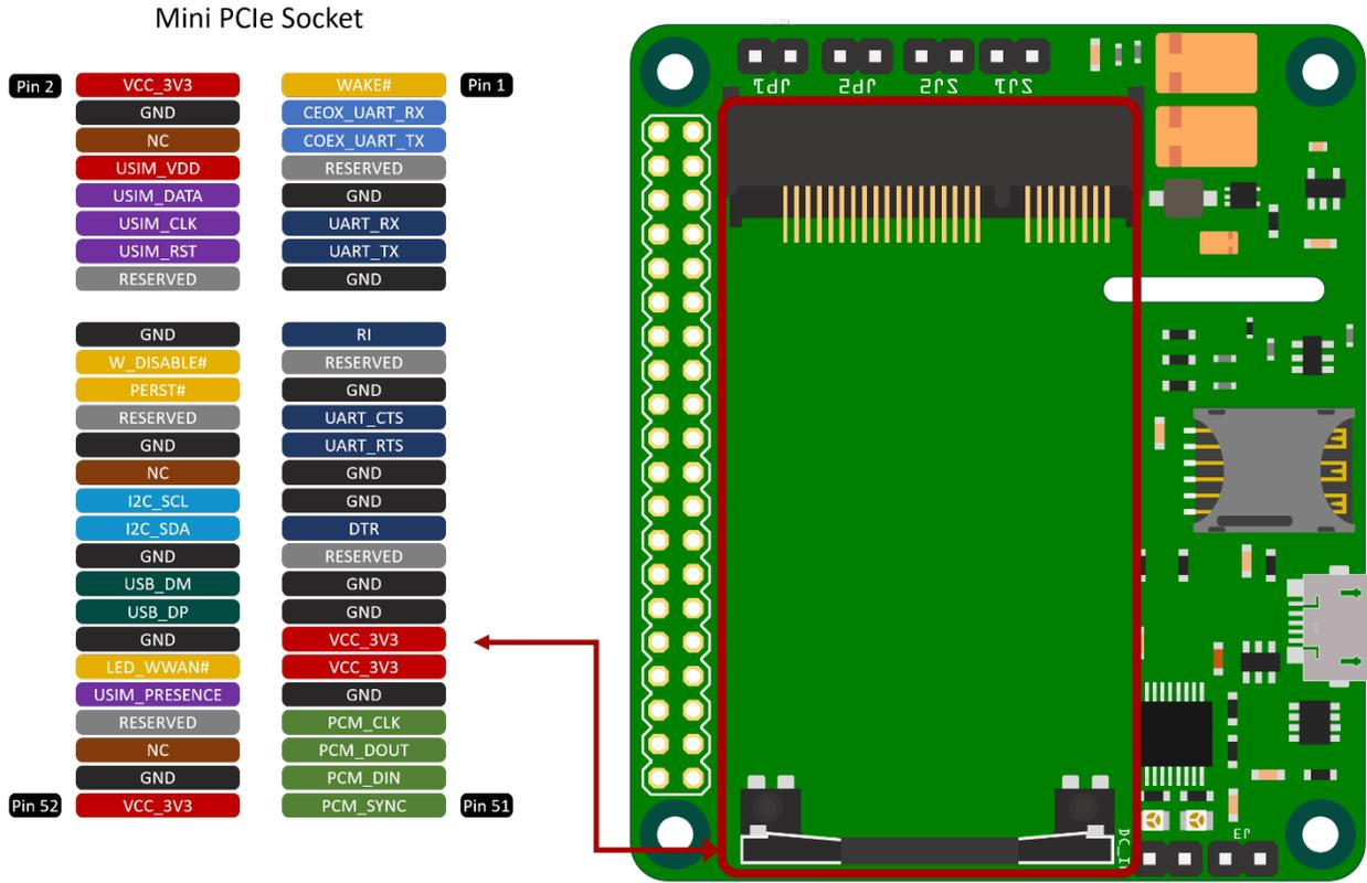
Figure 3. miniPCIe Pin Assignment
