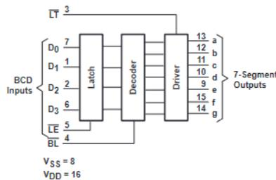
Figure 7-1. Function Diagram
