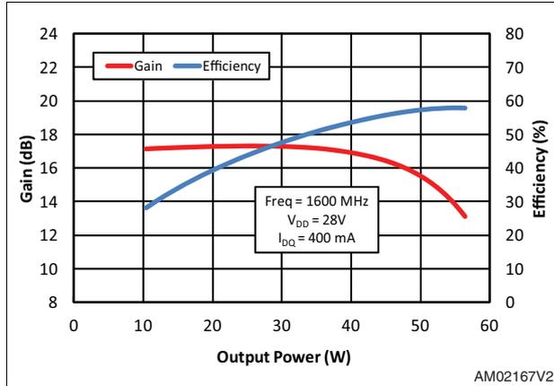
Figure 3. Gain vs output power and bias current
