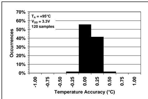
**FIGURE 2-2:** Temperature Accuracy Histogram,  $T_A = +95^\circ C$ .
