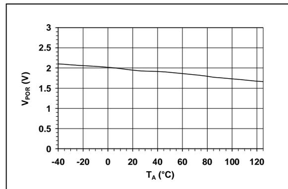
**FIGURE 2-6:** Power-on Reset Threshold Voltage vs. Ambient Temperature.
