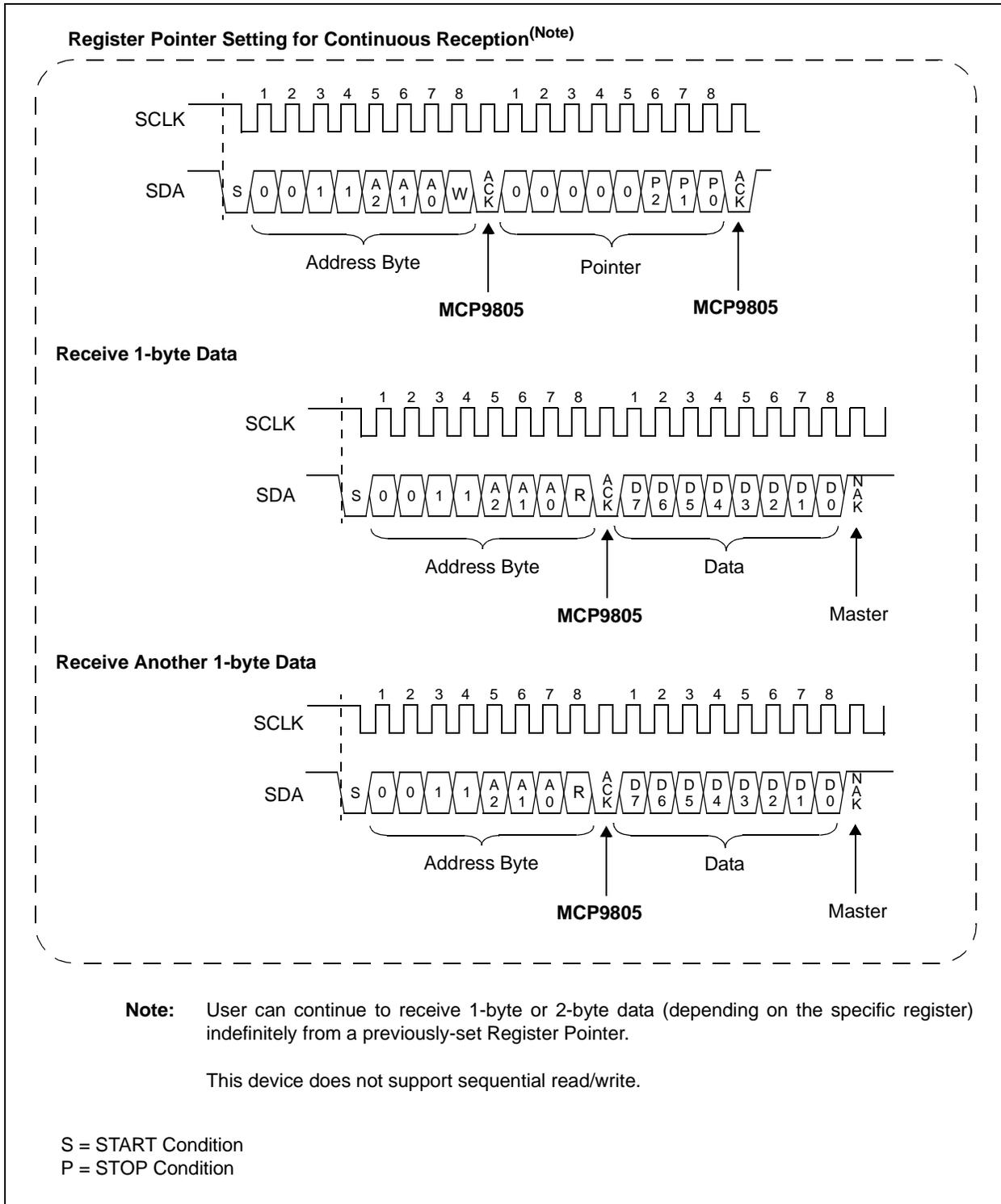
**FIGURE 5-4:** Receive 1-byte Data from Previously Set Pointer.
