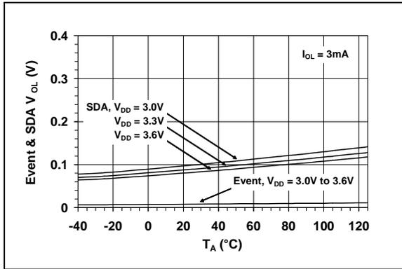
**FIGURE 2-7:** Event and SDA  $V_{OL}$  vs. Ambient Temperature.
