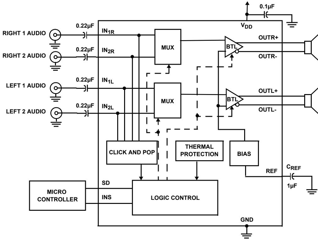
**ISL54002 Typical Application Circuit and Block Diagram**
