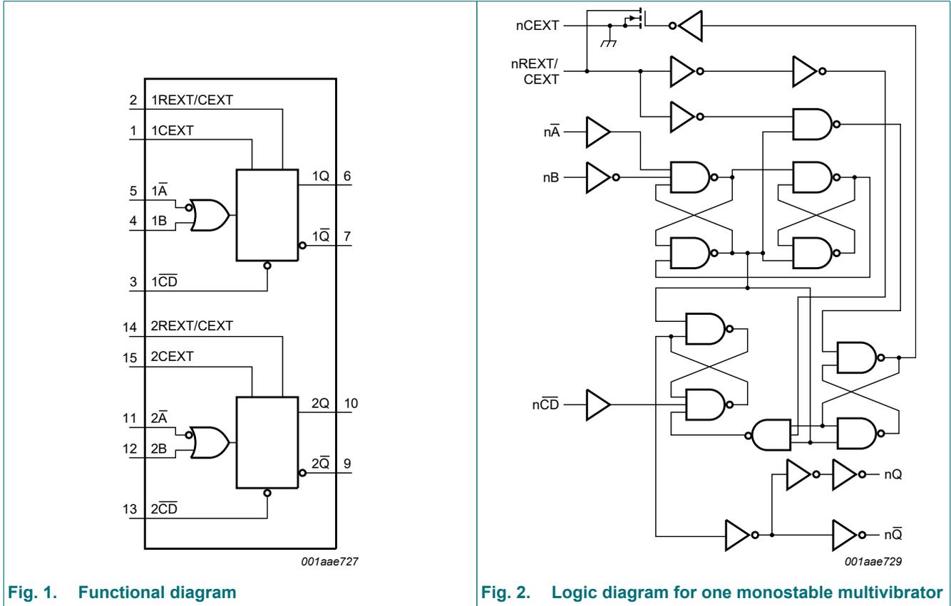
Fig. 1. Functional diagram
