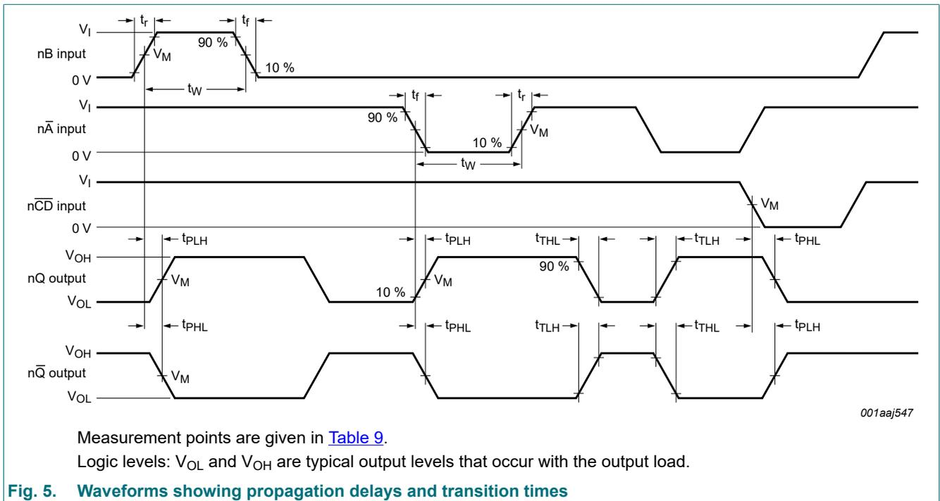
Fig. 5. Waveforms showing propagation delays and transition times
