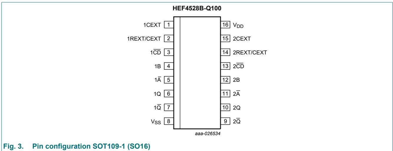
Fig. 3. Pin configuration SOT109-1 (SO16)
