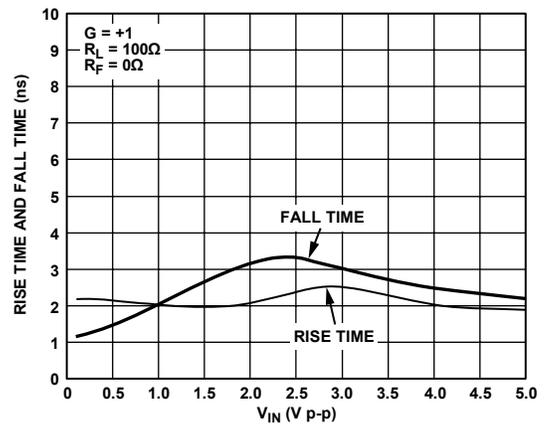
Figure 16. Rise Time and Fall Time vs.  $V_{IN}$
