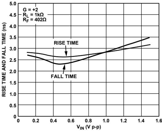
Figure 20. Rise Time and Fall Time vs.  $V_{IN}$
