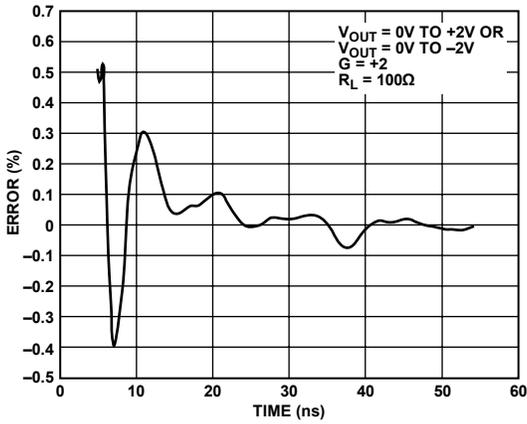
Figure 18. Settling Time
