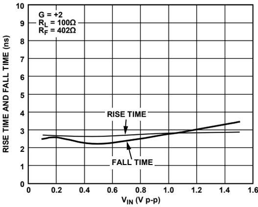
Figure 19. Rise Time and Fall Time vs.  $V_{IN}$
