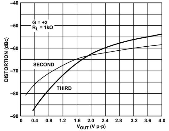
Figure 15. Distortion vs.  $V_{OUT}$  @ 20 MHz
