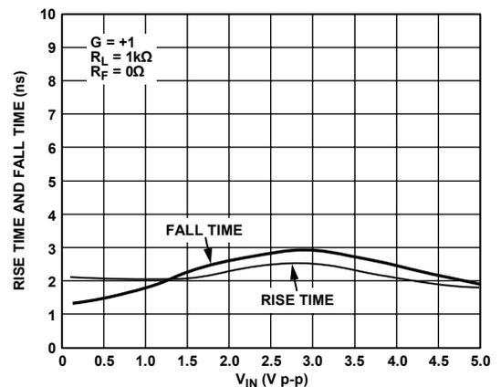
Figure 17. Rise Time and Fall Time vs.  $V_{IN}$
